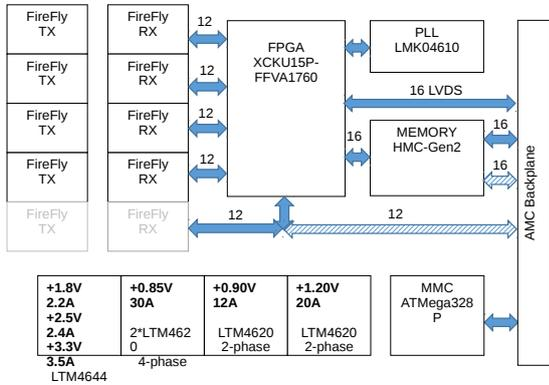
Figure 4.2: Block diagram of the PANDA Data Concentrator.
