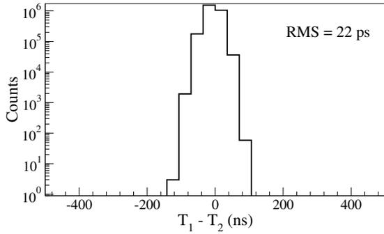
**Figure 4.15:** Measurement of the jitter induced by the measurement set-up.
