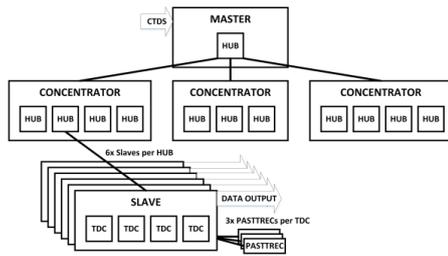
**Figure 3.12:** Readout architecture for the forward tracker in the High Resolution mode.
