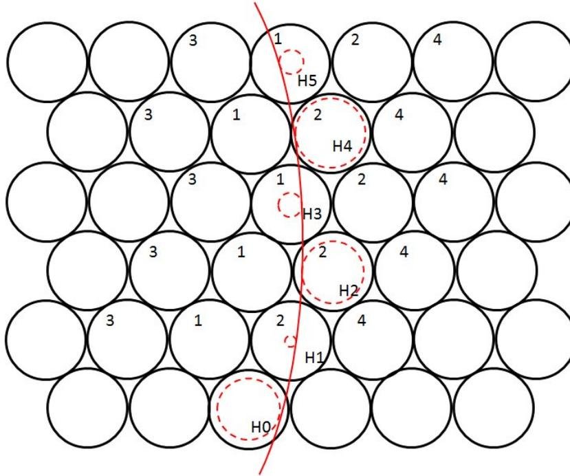
**Figure 4.29:** Illustration of the track finding algorithm. The black circles represent the individual straw tubes. The red solid curve indicates the trajectory of a charged particle. The red dashed circles inside tubes represent the isochrones.
