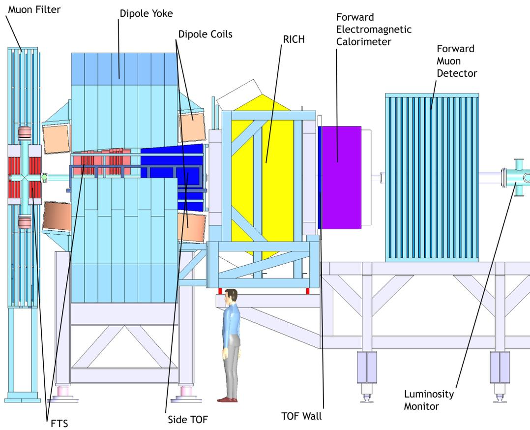
Figure 2.5: Side view of  $\bar{P}$ ANDA forward Spectrometer (FS). The antiproton beam enters from the left.
