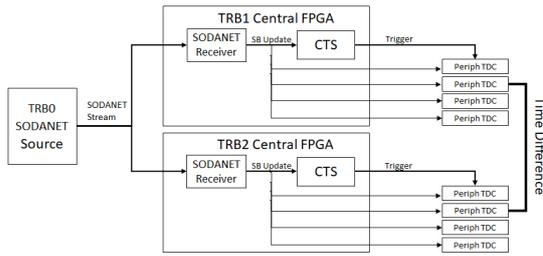
**Figure 4.21:** Hardware set-up used for long-term stability-tests of the SODANET synchronization protocol.
