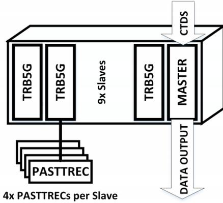
**Figure 3.13:** Readout architecture for the forward tracker in the High Luminosity mode.
