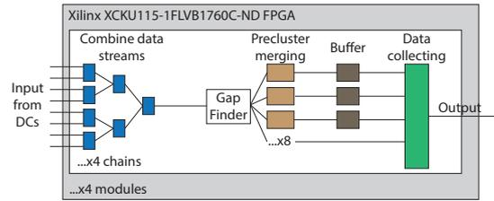
**Figure 4.46:** Block diagram of the FPGAs in the L1 nodes. Each FPGA has four modules, and each module has each four chains. One of the chains is shown. Each chain processes a different part of the data from the same eight inputs, based on their superburst number, but has its own output. Hence, the FPGAs use 32 inputs and 16 outputs. More details can be found in the text.
