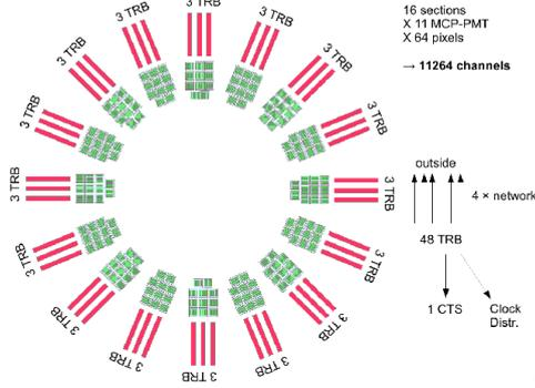
**Figure 3.10:** The readout structure of the barrel DIRC subsystem using TRB3 boards.
