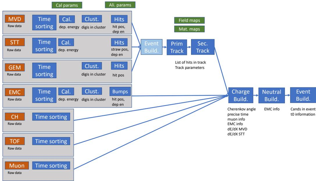
Figure 4.26: Schematic view of the data flow to the different processing stages within the PANDA experiment
