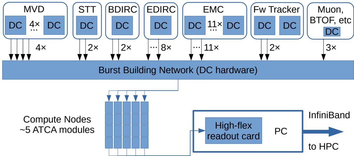
Figure 4.27: The overview of the PANDA readout system starting at the Data Concentrator (DC) level.
