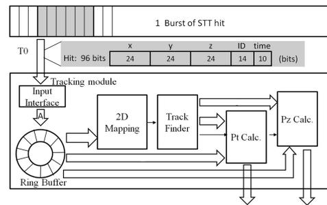
**Figure 4.32:** Simplified block-diagram of the algorithm in VHDL.
