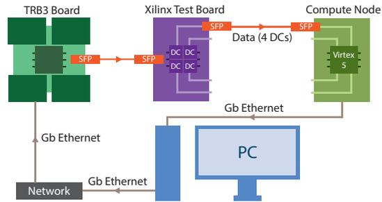
**Figure 4.44:** Schematic overview of the setup that was used to test the implementation of the double-pass cluster-finding algorithm on a prototype of the readout hardware. The Compute Node prototype has a Xilinx Virtex 5 FX70 FPGA with 11,200 slices and 5,328 kB RAM. The test board has a Xilinx Kintex 7 XC7K325 FPGA with 50,950 slices and 16,020 kB RAM. Further details are described in the text.
