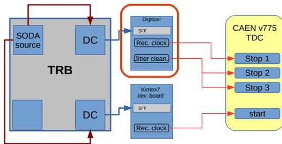
**Figure 4.16:** Scheme of the setup used for the long-term stability test of the SODANET.
