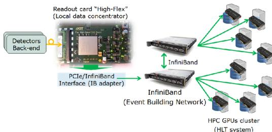
Figure 4.6: The basic concept of direct FPGA-GPU data-link tunnelled through InfiniBand network [1].
