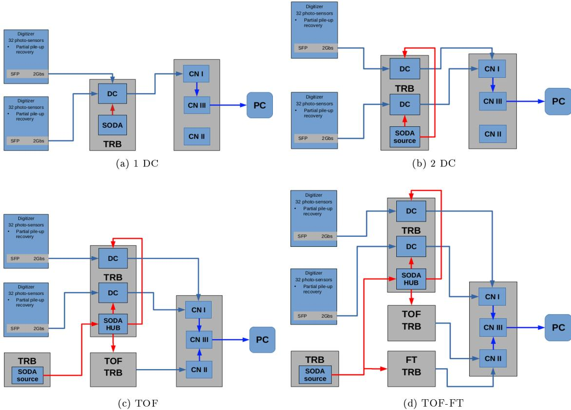
**Figure 5.7:** Diagrams of readout schemes which were tested during the beamtime at COSY. The top two, (a) and (b), were used for tests only with Proto9. The bottom diagrams represent the cases when other subdetectors were connected in addition to the EMC prototype.
