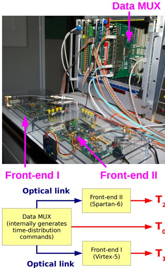
**Figure 4.12:** The photograph (upper panel) and a sketch (lower panel) of the set-up used to test the synchronous serial optical-link connection.
