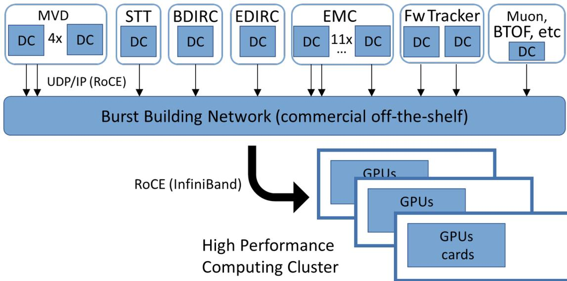
**Figure 4.28:** The overview of the PANDA readout system employing commercial hardware at the burst-building level.
