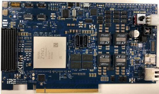
Figure 4.5: PCIe High-Flex readout card [1].
