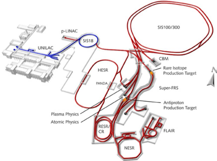
**Figure 2.1:** Schematic of the future FAIR layout incorporating the current GSI facilities on the left; on the right the future installations, the SIS 100 synchrotron the storage and cooler ring complex including CR and HESR and the Super FRS experiment being some of the new parts.  $\bar{P}$ ANDA is positioned right in the center of the image inside the HESR.
