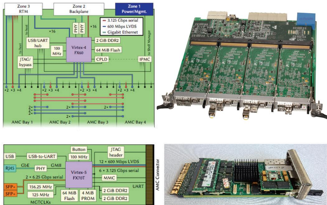
**Figure 4.4:** ATCA compliant FPGA based compute node. (top): carrier board; (bottom) xFP daughter board. The architecture is based on XILINX<sup>®</sup> Virtex FPGAs. A single CN can support up to 16 optical links and a total of 18 GB DDR2-RAM. The FPGAs are equipped with embedded PowerPC - CPUs, running Linux operating systems for slow control functions.
