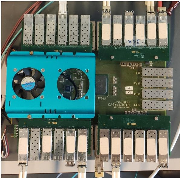
**Figure 5.6:** Photograph of the TRBv3 board. Two FPGAs on the right side perform functions of the DC. Another two on the left side: the top one is the UDP server, and the bottom one is the SODANET source.
