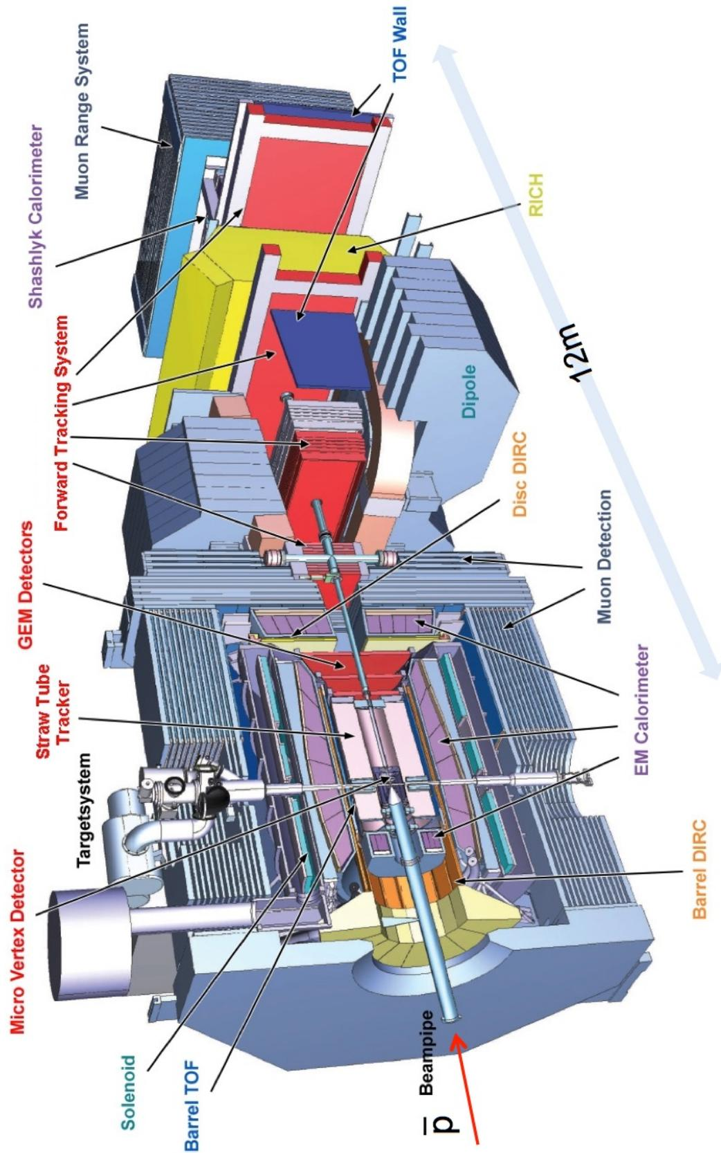
**Figure 2.3:** Aerial view of PANDA with the Target Spectrometer (TS) on the left side, and the Forward Spectrometer (FS) starting with the dipole magnet on the right. The antiproton beam enters from the left.
