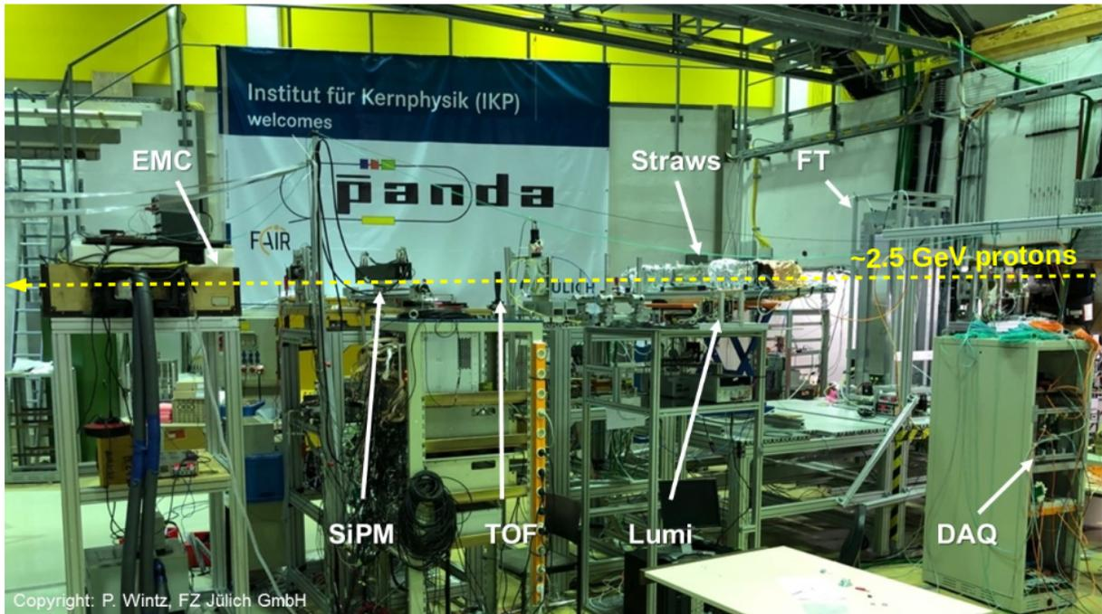
Figure 5.4: Final detector's setup during the testbeam time at COSY.
