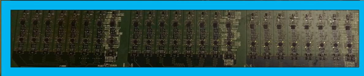
3 Scintillators X 8 discriminators per Scintillator = **24 channels**
