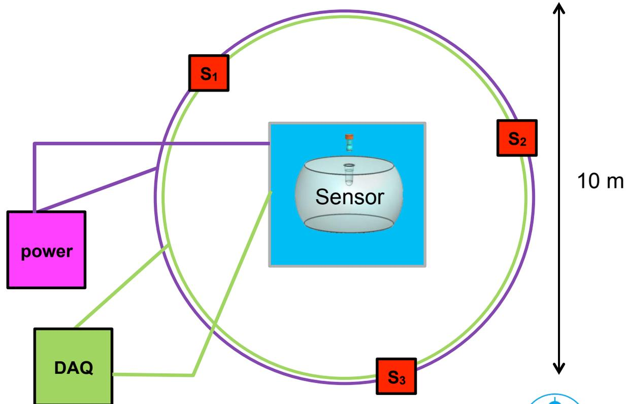
Reference detectors allow triggering and reconstruction of air showers!
