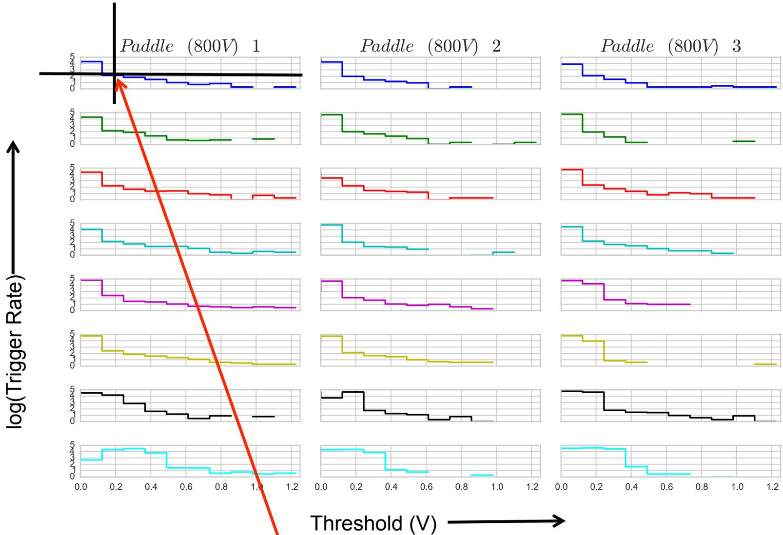
Set discriminator threshold via pre determined channel trigger rate
