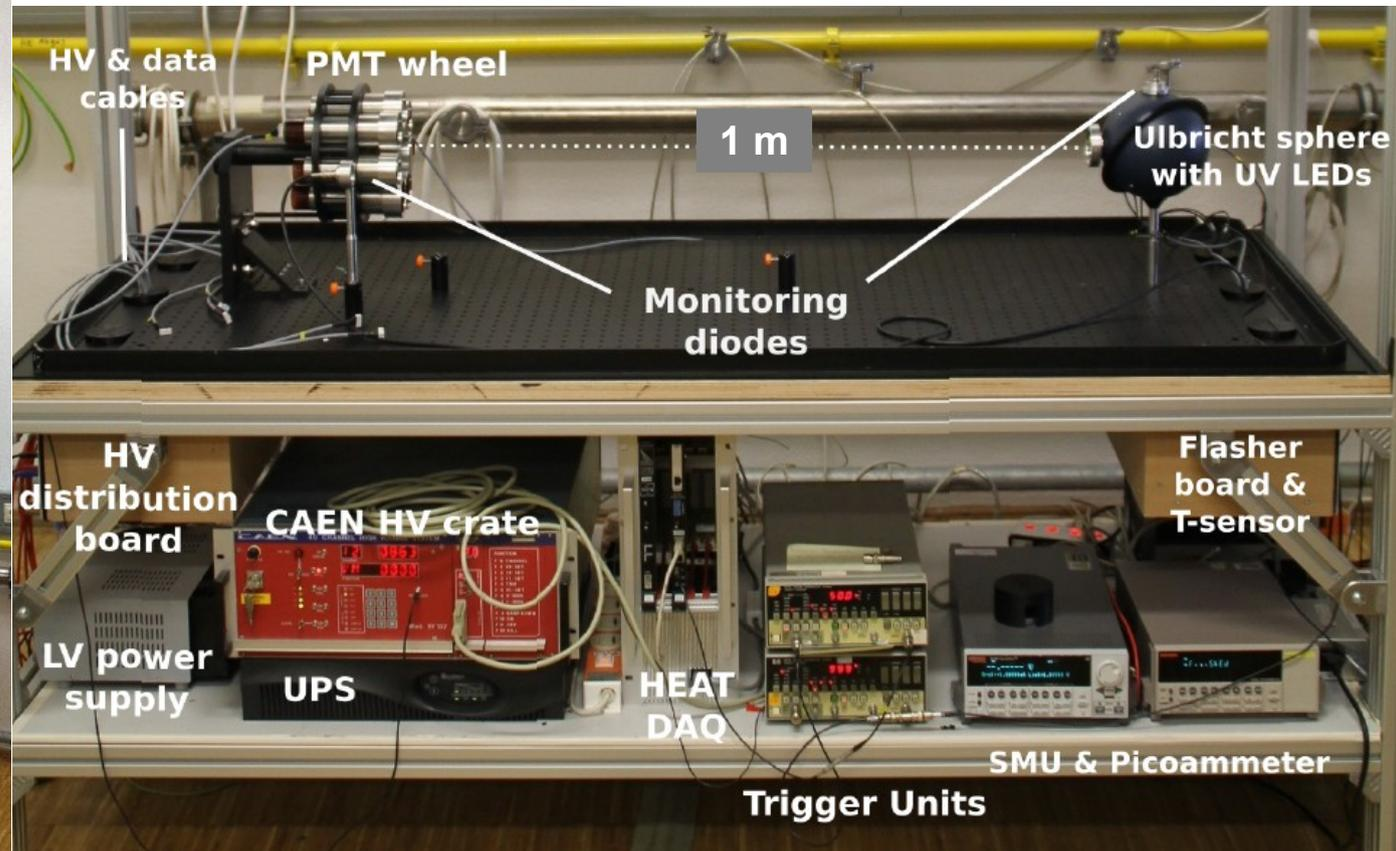
A uniform UV light source, which can be simultaneously operated in the DC and pulsed mode, illuminates FD PMTs. The FD electronics (20 MHz) is used to read-out measured signals.
