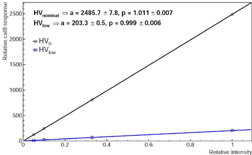
The camera averaged response to calib. B as a function of calib. B intensity for nominal HV (black circles) and reduced HV (blue squares).
