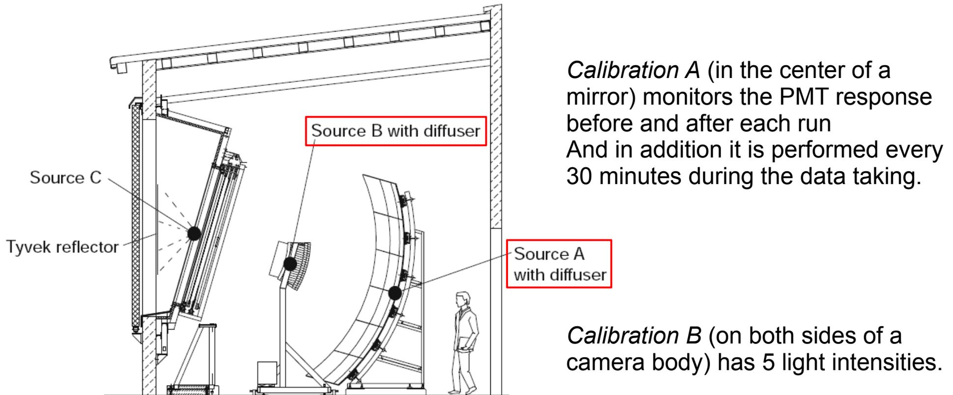
*Calibration A* (in the center of a mirror) monitors the PMT response before and after each run
