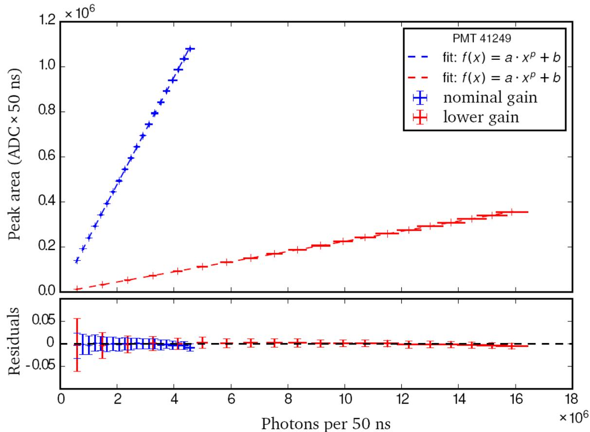
The PMT response to photon flux up to the saturation level measured at the nominal (blue) and reduced (red) gain. The exponent  $p$  is 1.0 for both gains.
