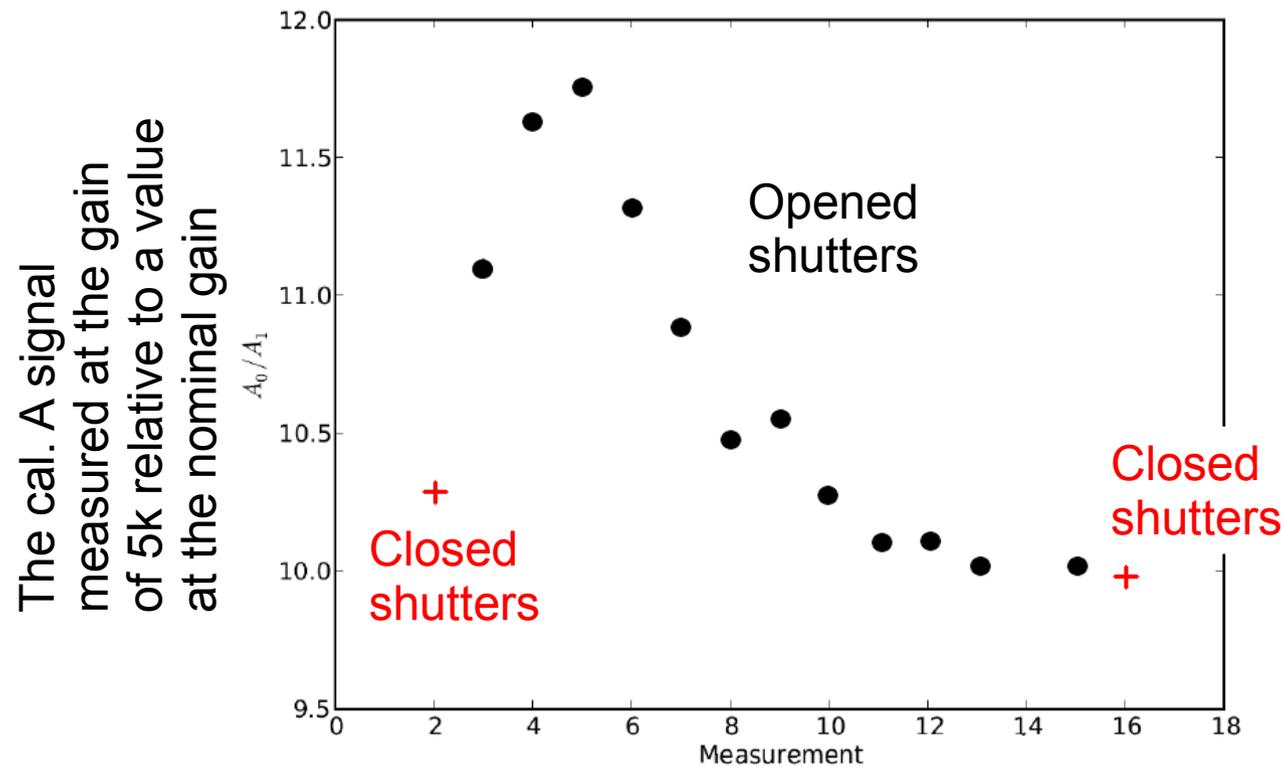
Figure 6: The relative response of the PMTs measured at the reduced gain during data taking. Crosses and stars indicate closed and open shutters, respectively.
