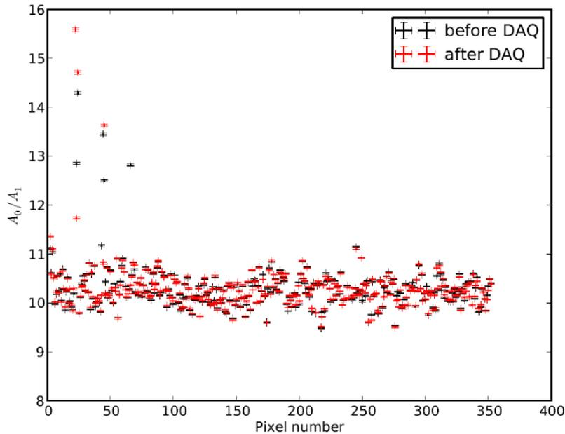
The ratio of calib. measurement A at the nominal ( $5 \times 10^4$ ) and reduced gain ( $5 \times 10^3$ ) before (black) and after (red) data taking.
