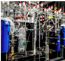
Gas line for Rn measurements
