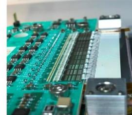
Figure 13. The 384-strip germanium detector wire-bonded to 12 MARS ASICs.
