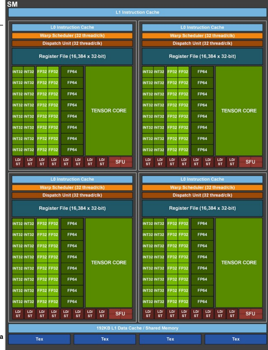
Figure 5. The GA100 streaming multiprocessor (SM).
