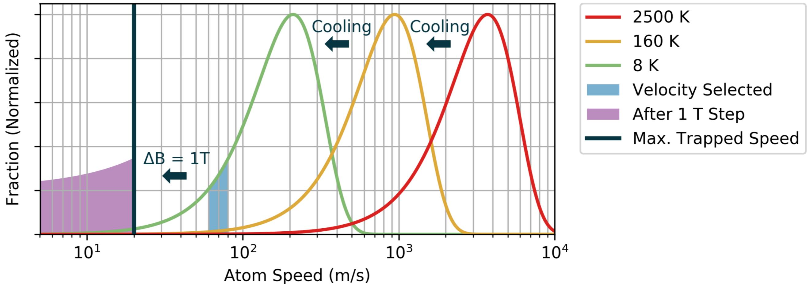
Magnetic field step into solenoid
