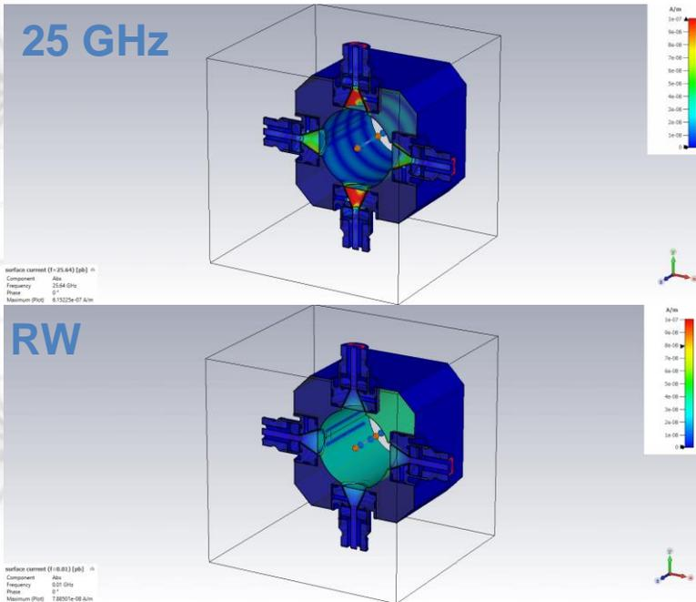
Beam induced surface current at 25 GHz (top) and at low frequency (bottom). SOLEIL CST simulation.
