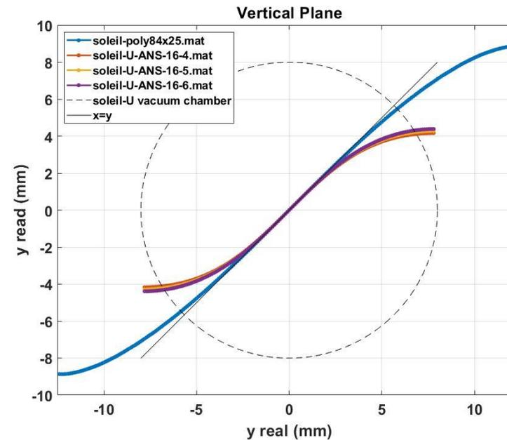
Delta over Sum response  $\Phi 16$  mm BPM. Linear region is  $\pm 2$  mm. *BPMLab simulation [1].*
