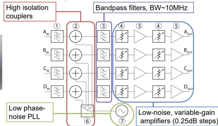
Pilot Tone front-end developed at Elettra. [G. Brajnik, IBIC 2018 \[10\]](#)
