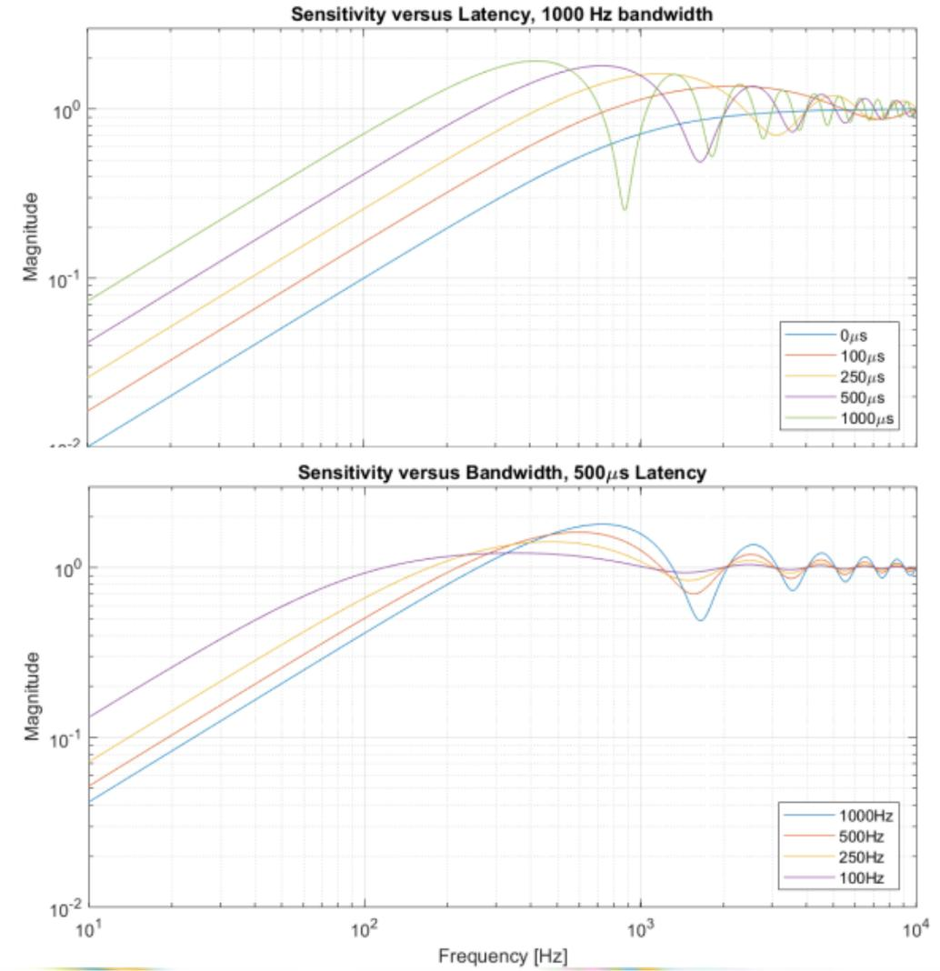
Influence of the latency and bandwidth on the feedback close loop response (with IMC controller).
