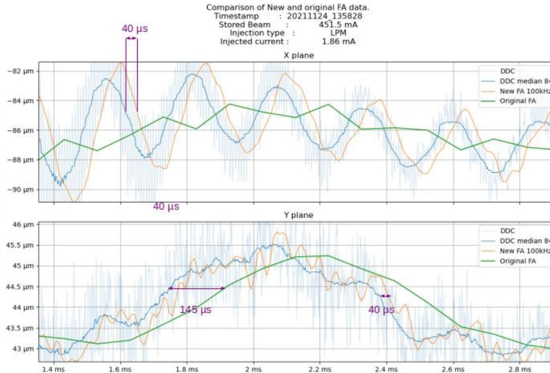
Numerical filtering of the TbT data by a 25 kHz butterworth filter compared with the current 2 kHz FIR filter . SOLEIL simulation.
