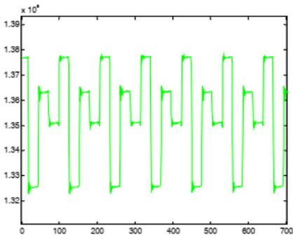
Figure 20: TBT data, one channel. Acquisition only with Switching Enabled. The Transitions between Four Switch Positions are Visible.
