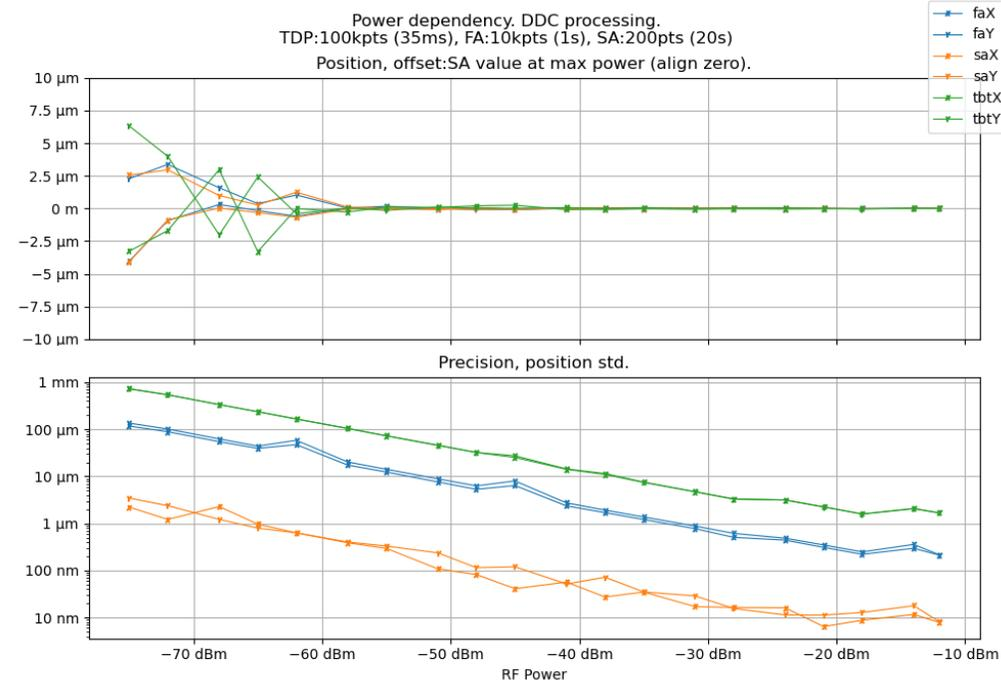
BCD and resolution lab measurement on a Libera Brilliance + BPM electronics for a 25% simulated filling pattern and a geometric factor of 11.4 mm (SOLEIL).
