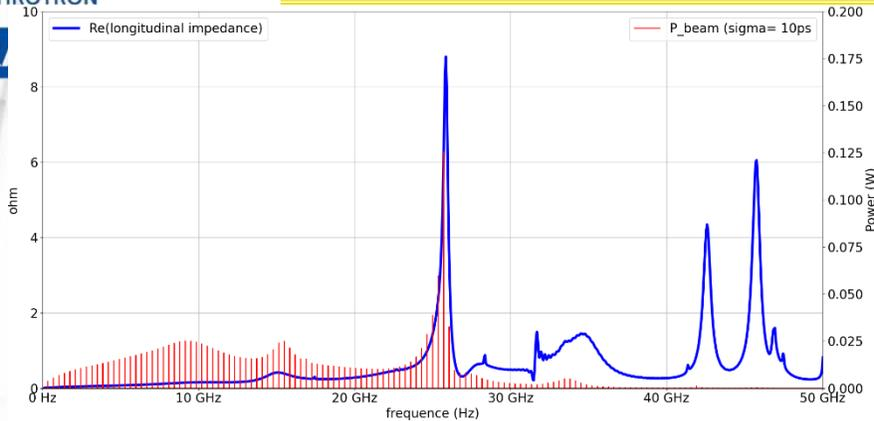
Real part of the long. Impedance (blue) and loss map (red) for a 10 ps rms bunch length (SOLEIL case)
