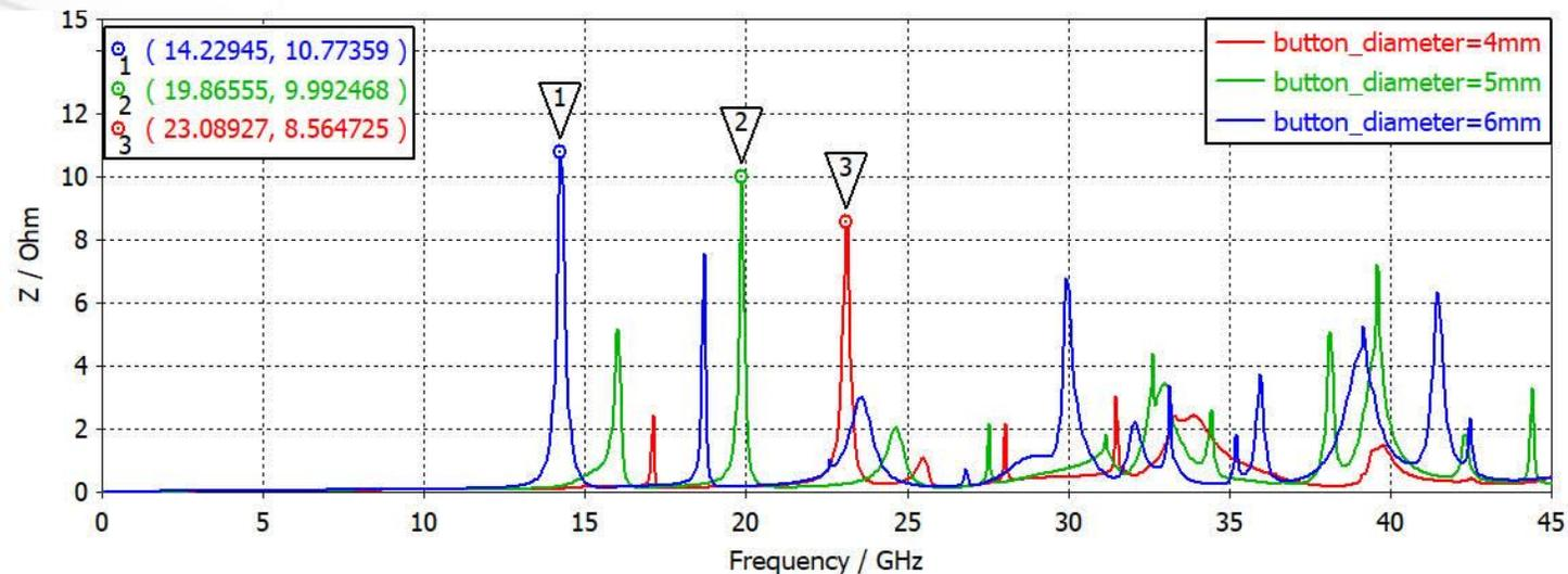
Longitudinal impedance (real part) vs. button diameter. SOLEIL simulations. [M. El-Ajjouri, IBIC2021 \[2\]](#)
