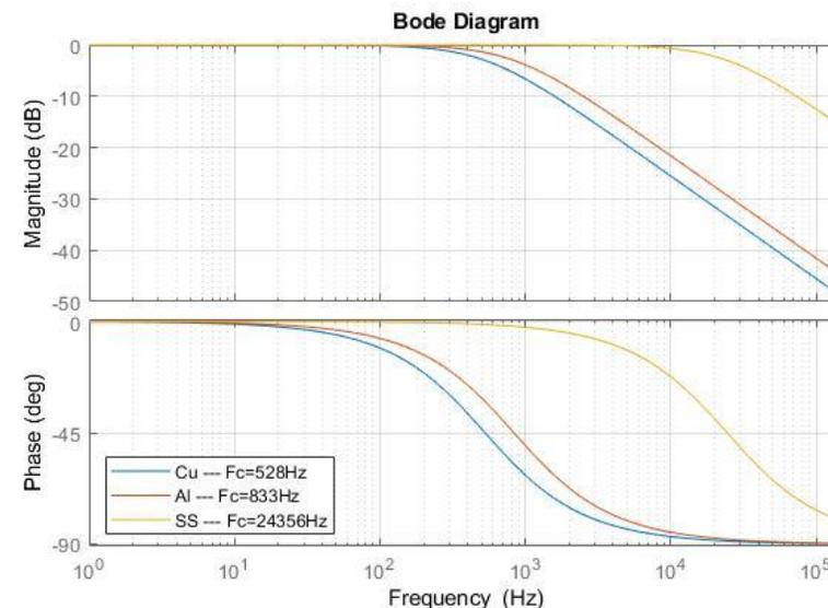
Gain and phase response of a 1 mm thick, 16 mm diameter circular vacuum chamber.
