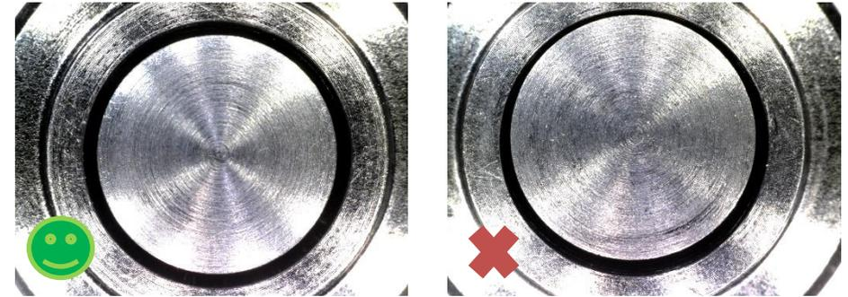
Control of the button gap (200 $\mu$ m) and concentricity with a microscope (SOLEIL prototype).
