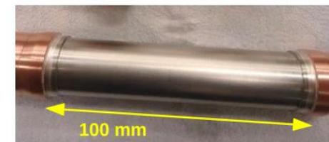
SIRIUS fast correctors vacuum chamber. The 0.3 mm SS circular geometry gives a cut-off frequency of 48 kHz [8]
