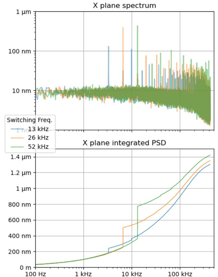
Turn by turn power spectral density for different switching frequencies. *SOLEIL test*
