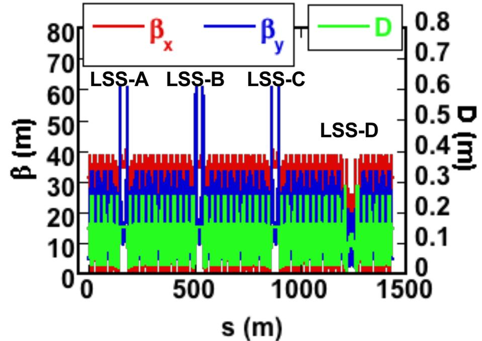
“SPring-8” = 44 x “unit cell” + 4 x “30m long straight section (LSS)”.
