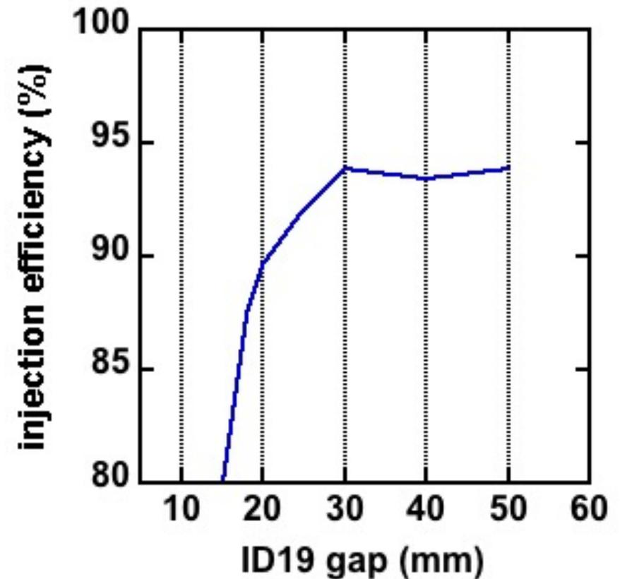
The tune shift caused by closing the gap of ID19 was not corrected.
