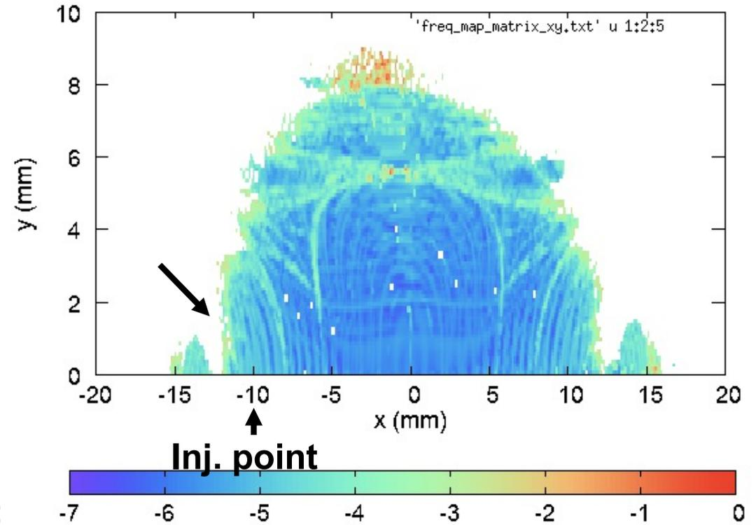
The unstable area induced by the resonance of  $3Q_y \sim \text{int.}$  is away from the injection point.
