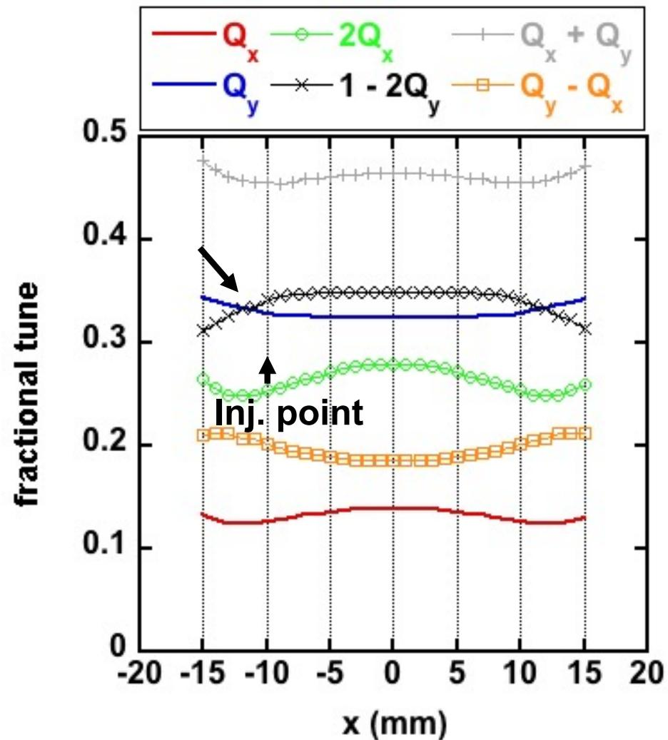
The resonance of  $3Q_y = \text{int.}$  is away from the injection point.
