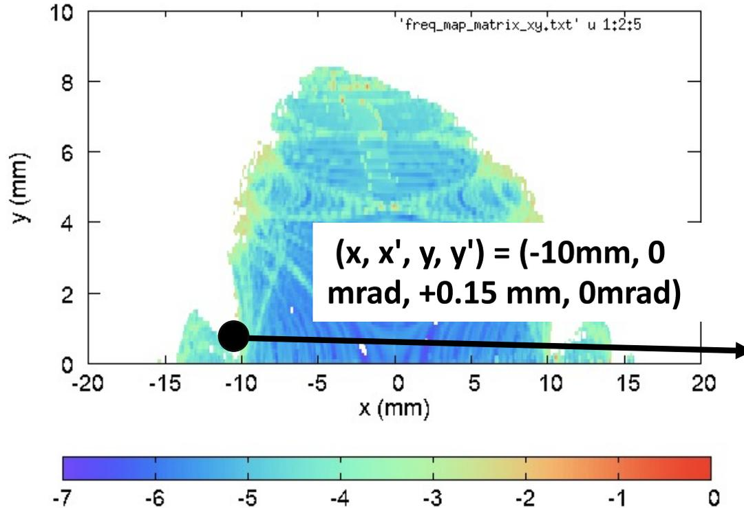
It seems that there is the unstable area around the injection point, **which is caused by the resonance of  $3Q_y \sim \text{int.}$** , and that a part of the initial beam is located at this unstable area.
