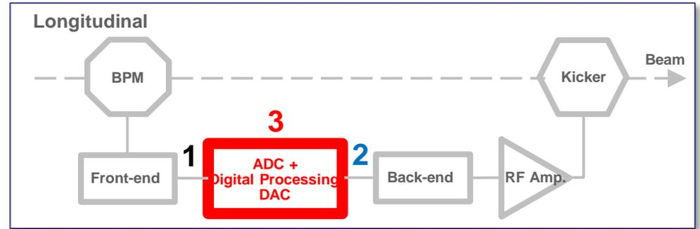
By means of a **sinusoidal digital filters** (16 taps), we obtain the **correction signal** for the **n-th bunch**. In first approximation, **the filter applies a gain** (user-selectable) and a **phase shift of  $-\pi/2$**  to the digitized signal.
