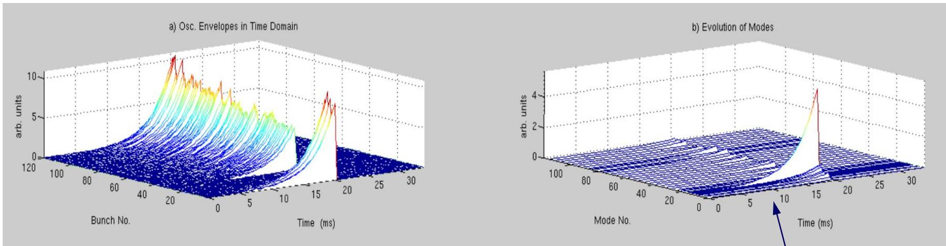
An example of the measurement performed with the longitudinal feedback on positron beam (100 bunches) with  $I_{avg} = 730$  mA
