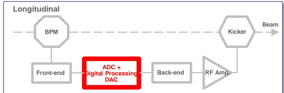
It represents the core of the system. It elaborates the correction signal, based on the phase measurements.
