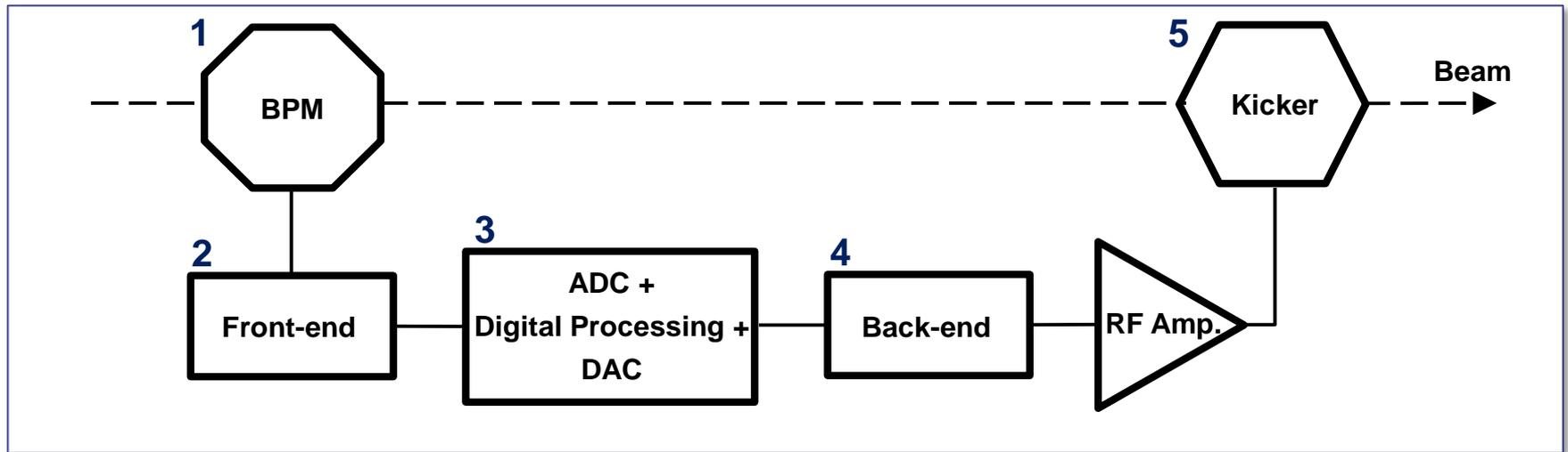
**The longitudinal feedback acts on the phase of the bunches.** It applies a correction signal in the form of a longitudinal kick (by means of a RF cavity).
