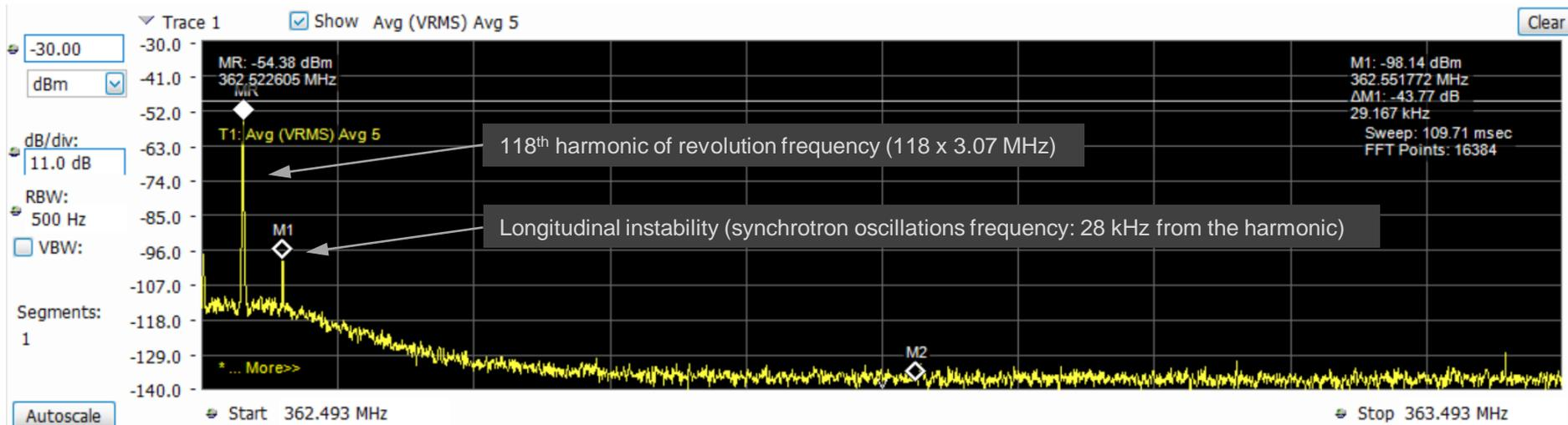
Example of beam spectrum with Positron beam (100 bunches) with  $I_{\text{avg}} = 150$  mA. Long. feedback turned off.
