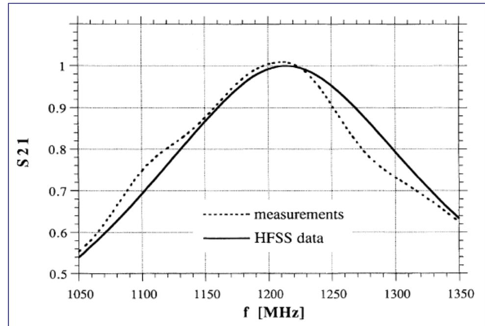
(see: A Waveguide overloaded Cavity as Longitudinal Kicker for the DAFNE Bunch-by-bunch feedback system. R.Boni, A.Gallo, A.Ghigo, F.Marcellini, M.Serio, M.Zobov. Particle Accelerators, 1996, Vol.52, pp 95-113)
