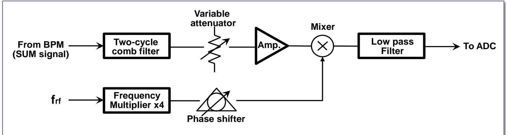
Variable attenuator and phase shifters values are controllable via software.
