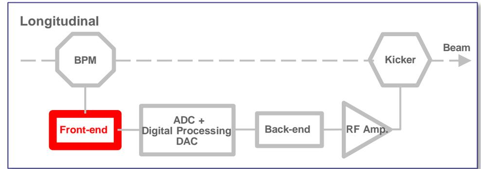
The Front-end main functionality is to transform the phase of the BPM signals into an amplitude signal (to be digitized later on).
