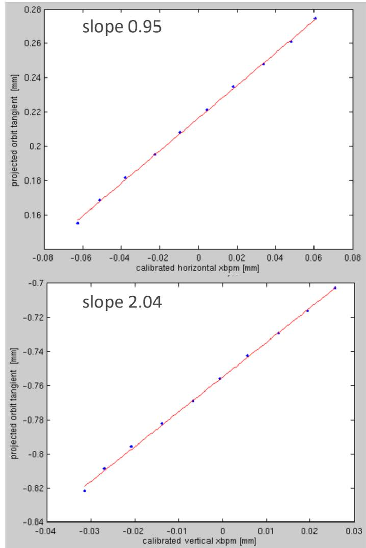
xbpm-measured vs expected photon beam position during a scan of orbit angle through an ID:
