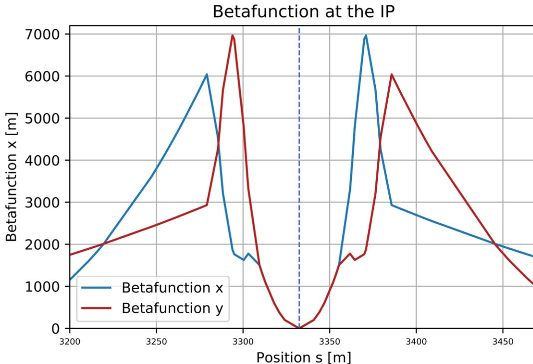
Betafunction before a drift space of the length  $l$  with **minimum betafunction  $\beta^*$**  :
