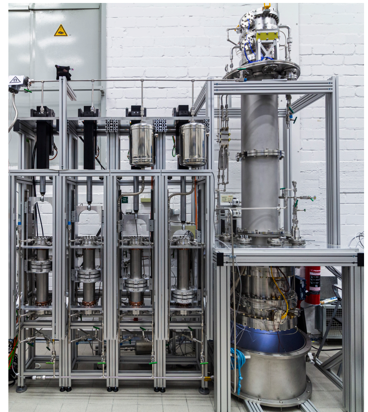
Rn distillation column (reduce ^{222}\text{Rn} - hence also ^{214}\text{Bi} - from pipes, cables, cryogenic system)
