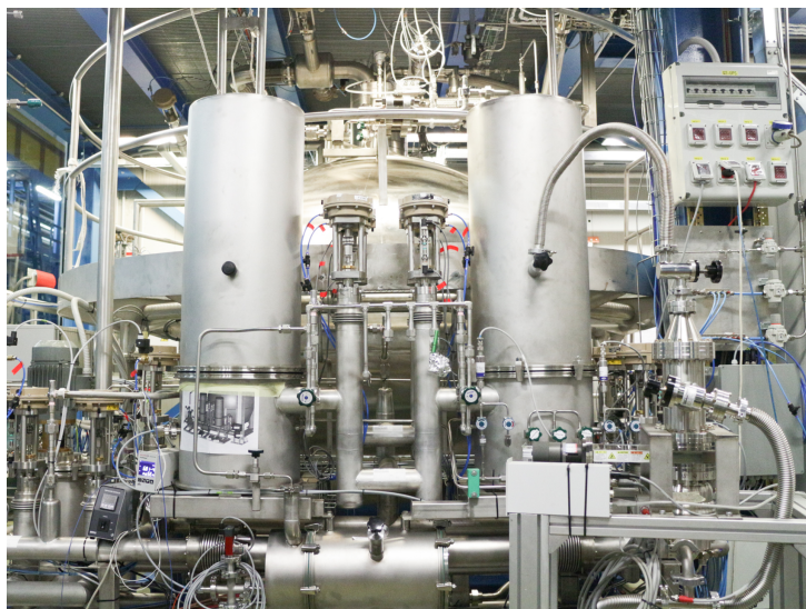
LXe purification system (5 L/min LXe, faster cleaning; 2500 slpm)
