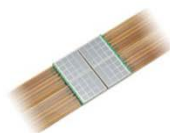
4x4ch monolithic array with FPC (15 cm) buttonable S11829-3344MF
