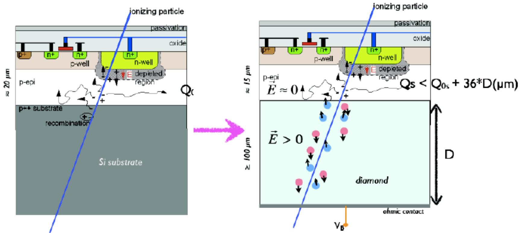
Si MAPS chip thinned to  $20\mu\text{m}$  from the rear side and bonded to a (biased) diamond plate.
