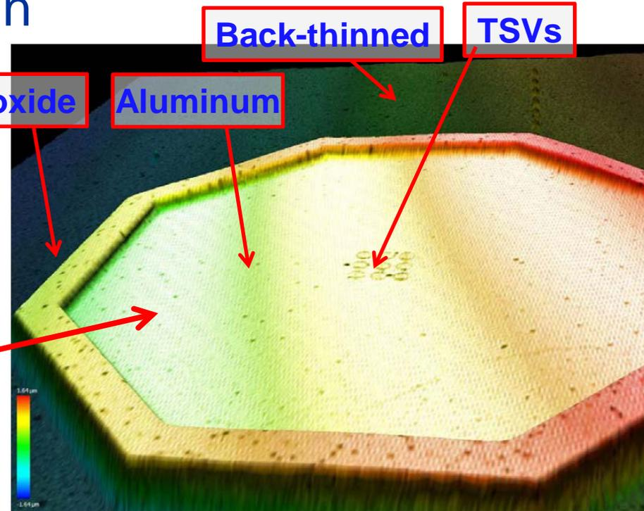
Fully finished 3D wafer (March 2013) Cu-Cu TC
