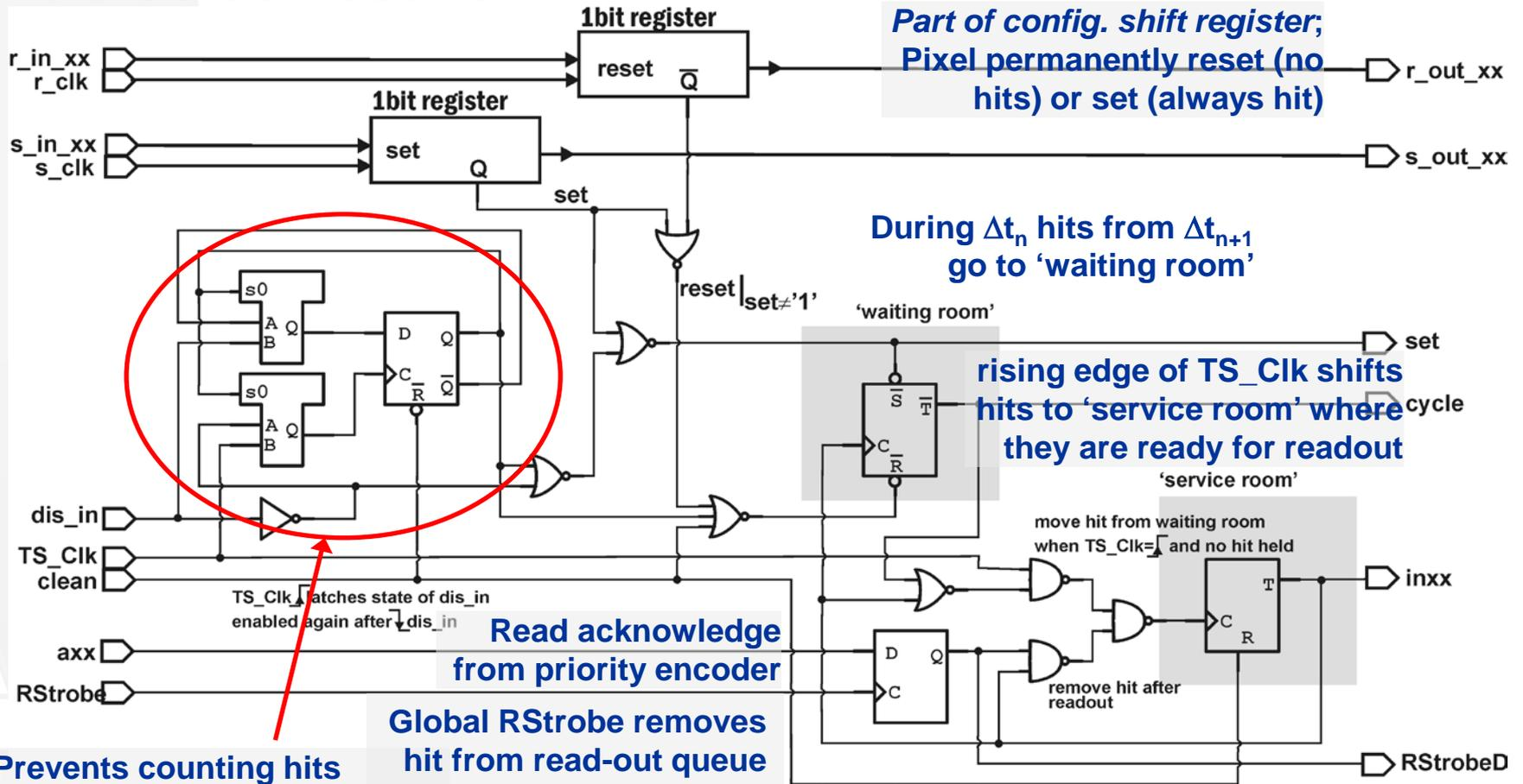
Demonstration of hit spilling between adjacent time slots
