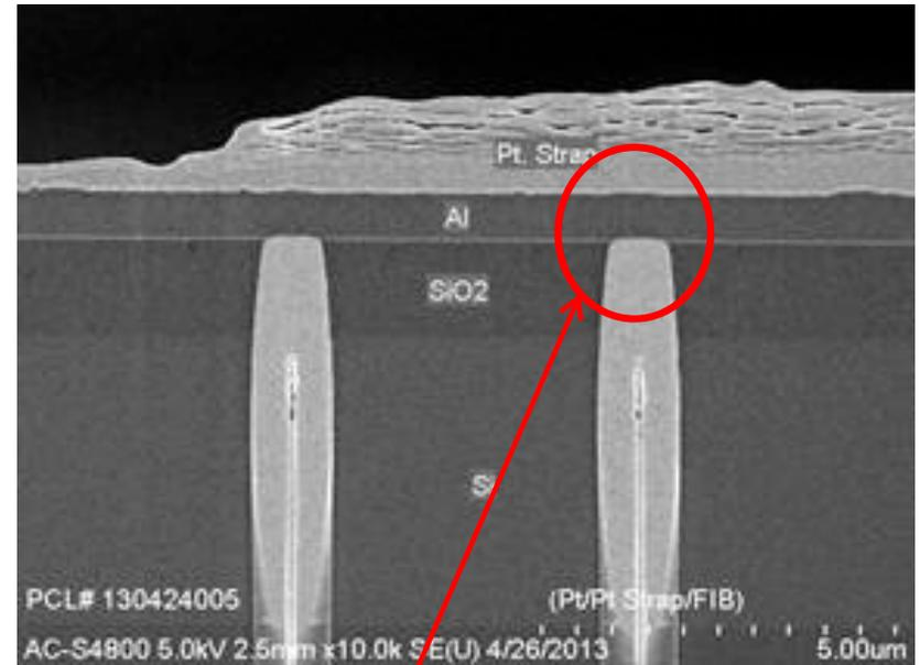
SEM image of W TSVs providing contact to back-side Al pad on VIPIC1
