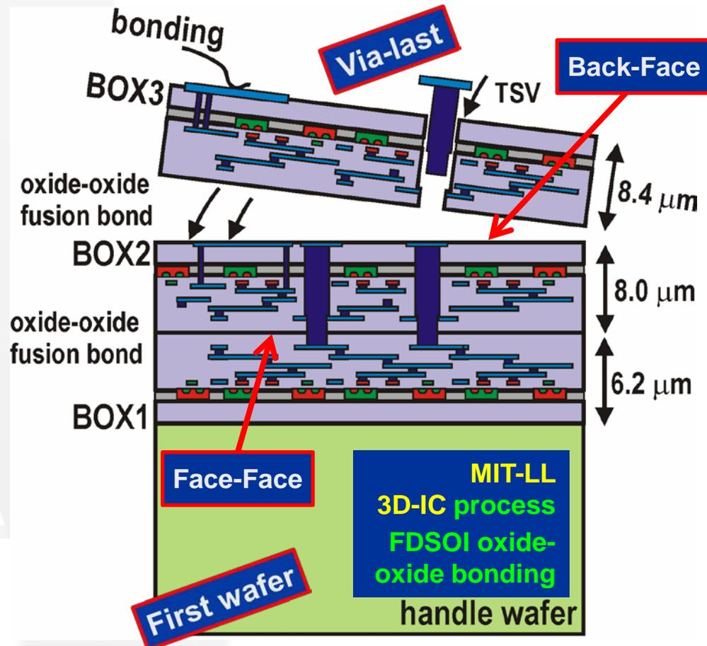
Technology option based on VIA LAST and SOI wafers
