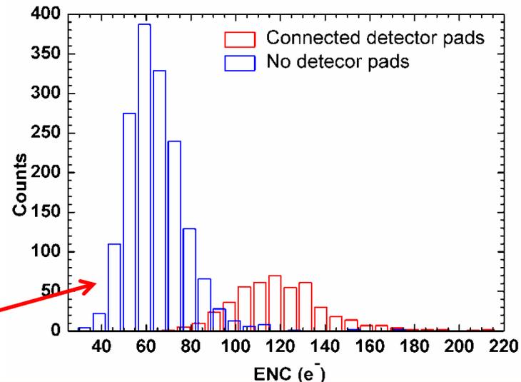
noise @ nominal bias in input transistor and with CSA replica off for gain from measurements
