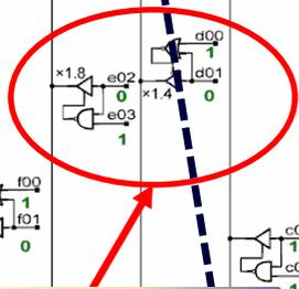
Logic (with tri-state capability) for generation of binary addresses
