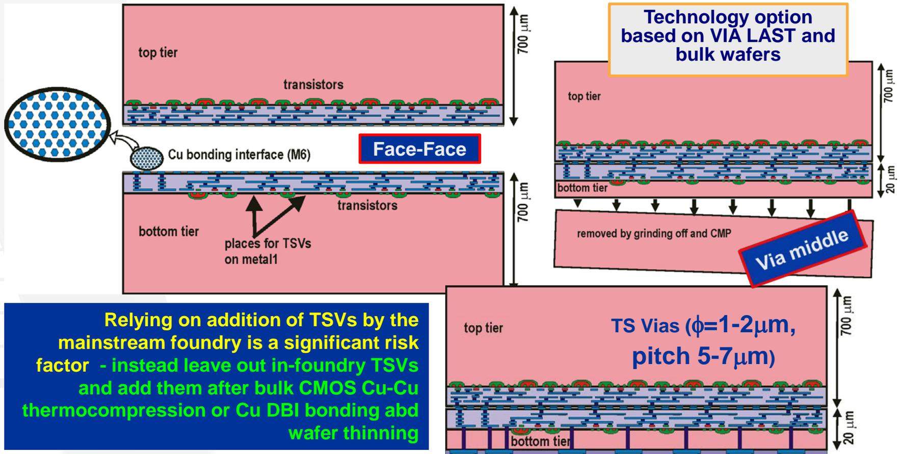
Relying on addition of TSVs by the mainstream foundry is a significant risk factor - instead leave out in-foundry TSVs and add them after bulk CMOS Cu-Cu thermocompression or Cu DBI bonding and wafer thinning
