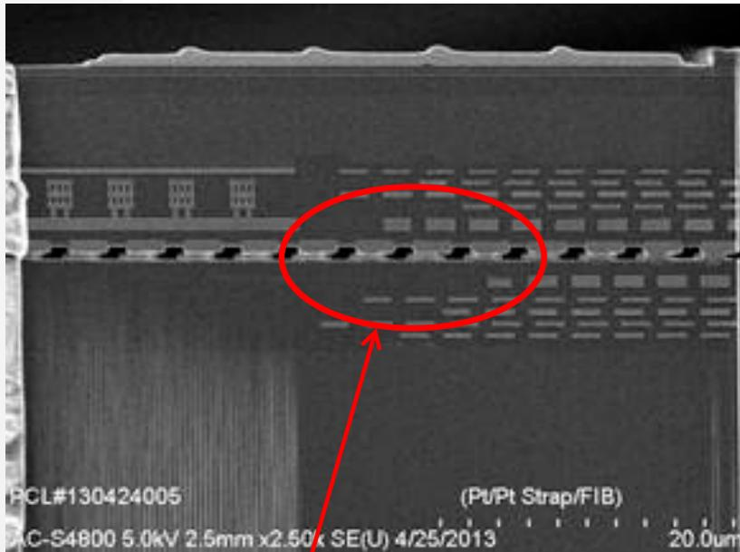
SEM image of Cu-Cu TC bonding interface on VIPIC1 acceptable alignment tolerance  $3\sigma < 1.2\mu\text{m}$
