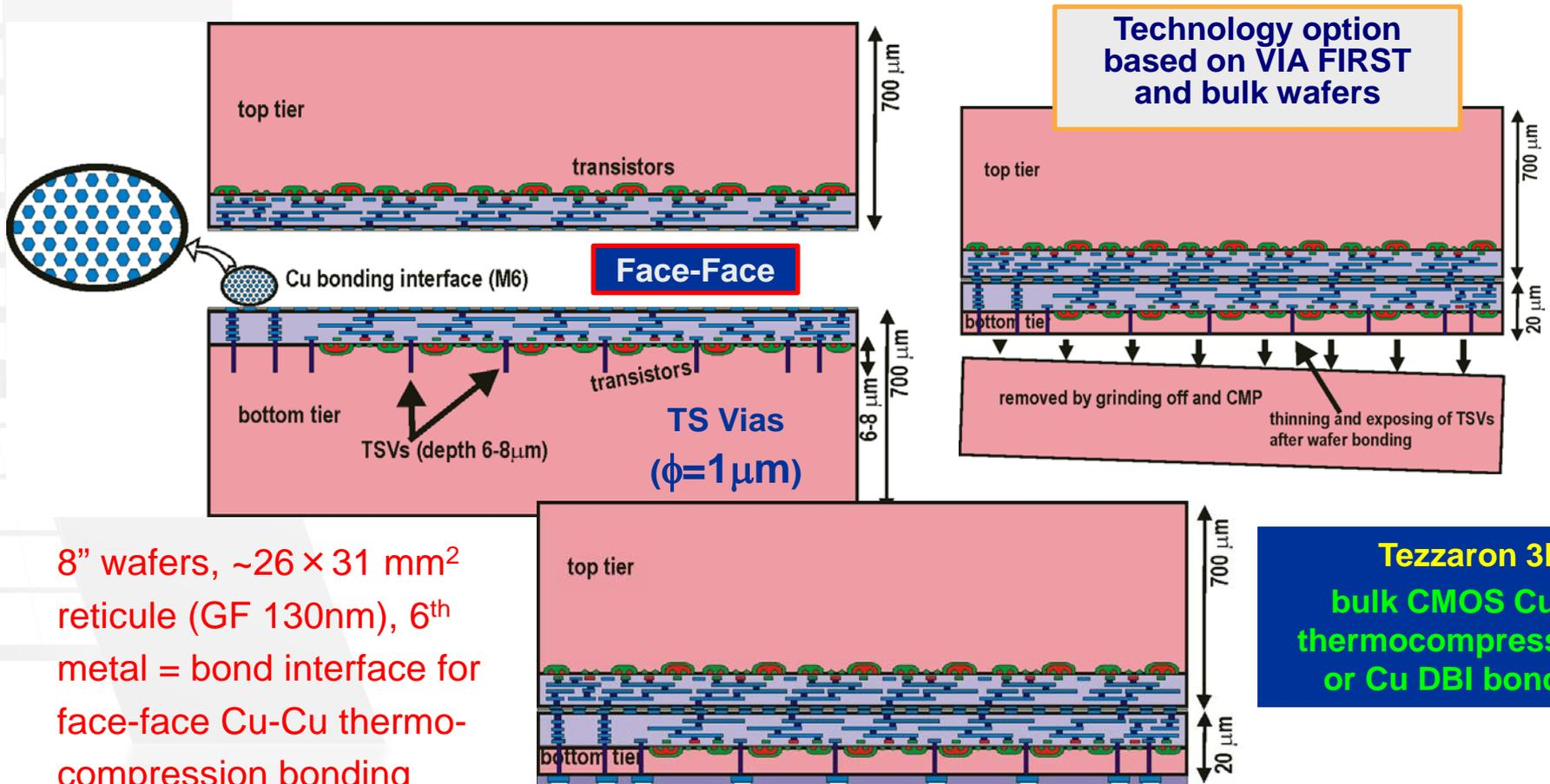
8" wafers, ~26 × 31 mm<sup>2</sup> reticule (GF 130nm), 6<sup>th</sup> metal = bond interface for face-face Cu-Cu thermo-compression bonding
