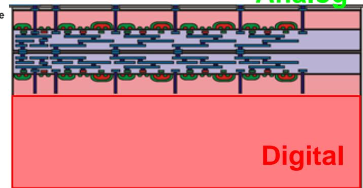
• **Analog** accessed directly, **Digital** must pass through bonding interface between tiers
