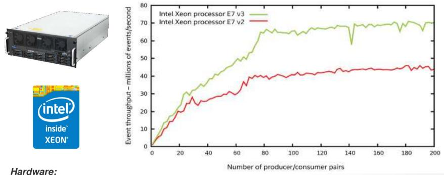
Intel Xeon processor family: 4 sockets, 18 cores per socket, Hyper-threaded, Xeon E7-8890 v3 CPUs
