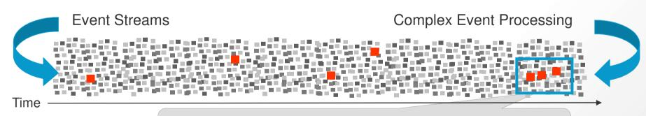
Complex Event Processing: "When more than 3 temperature events are received above a threshold, alert."
