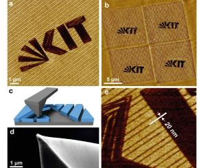
AFM topography with a z-range of 3 nm. Brush molecules were removed by applying a normal force of 1  $\mu$ N to the tip of the AFM, No broadening of the linewidth of 20 nm (FWHM) was observable within the accuracy of the measurement.
