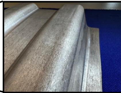
Component without surface defects
