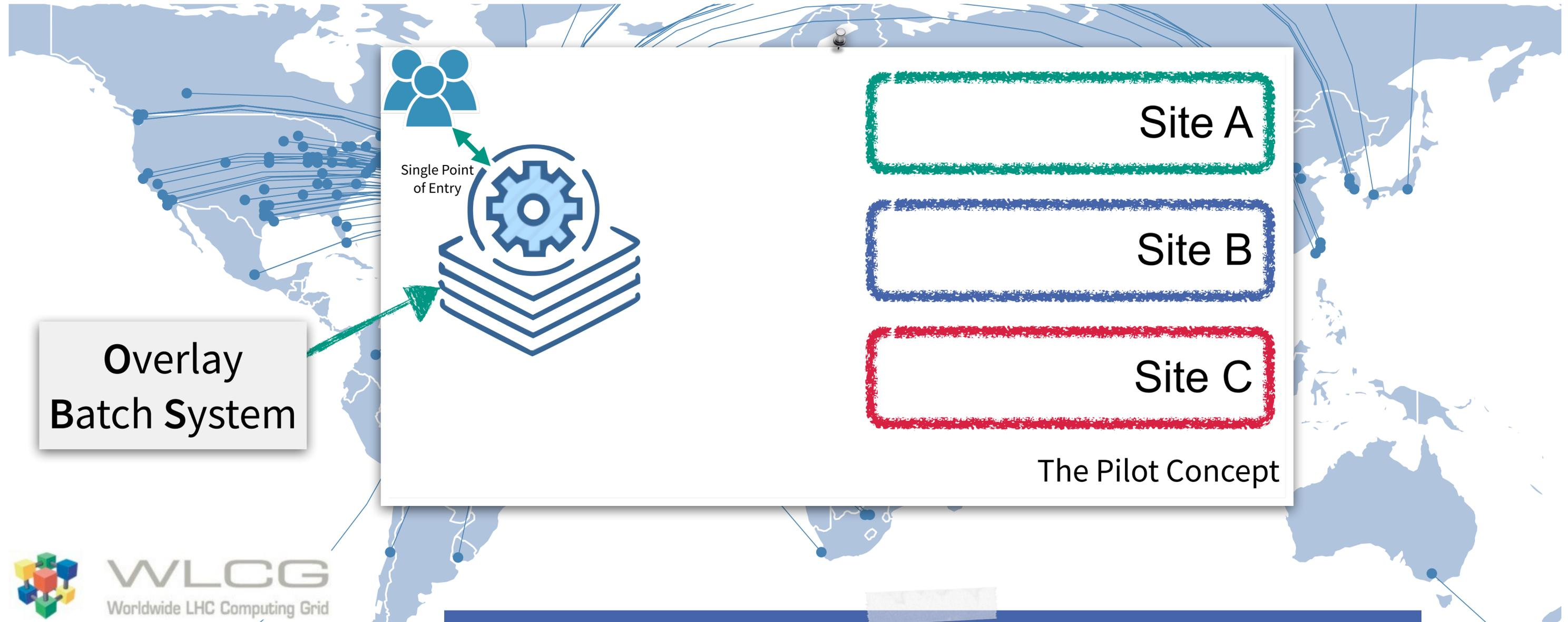
Integrate resources into a globally distributed batch system and remove some parts of the initial Grid middleware
