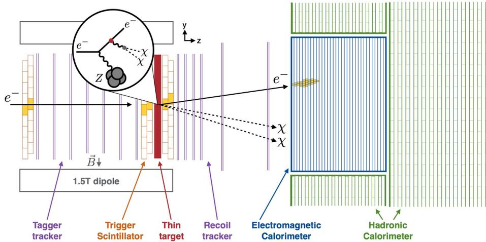
**Beam which enables  $O(10^{16})$  electrons to be individually identified & reconstructed**
