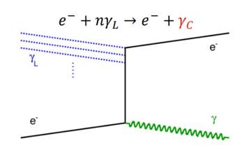
16.5 GeV electron, 800 nm laser, 17.2° crossing angle
