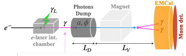
Photons produced in the e-laser collisions are freely propagating to collide with the nuclei of the material of the dump
