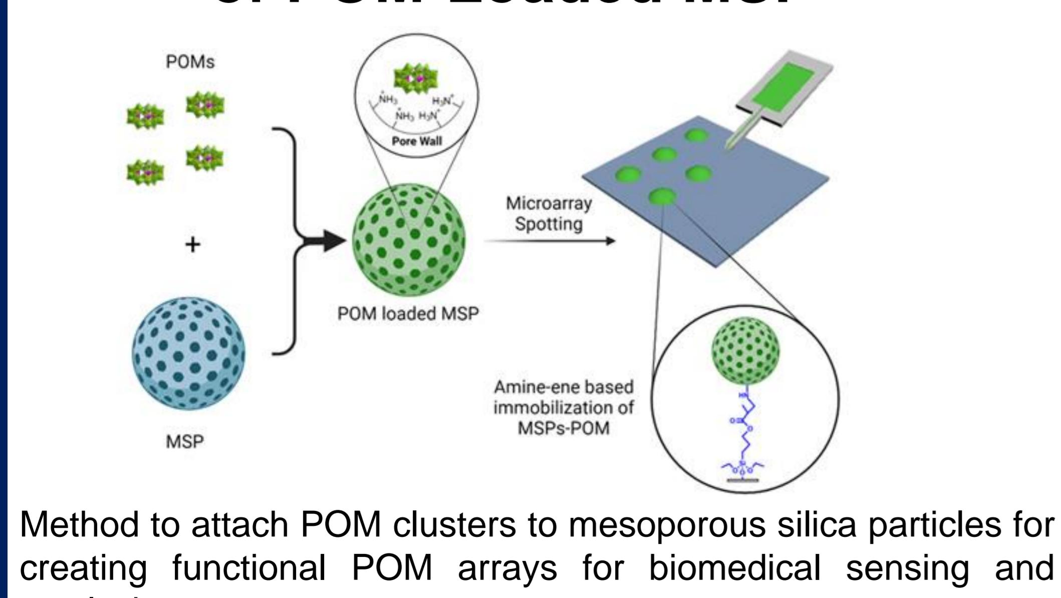
Method to attach POM clusters to mesoporous silica particles for creating functional POM arrays for biomedical sensing and catalysis.
