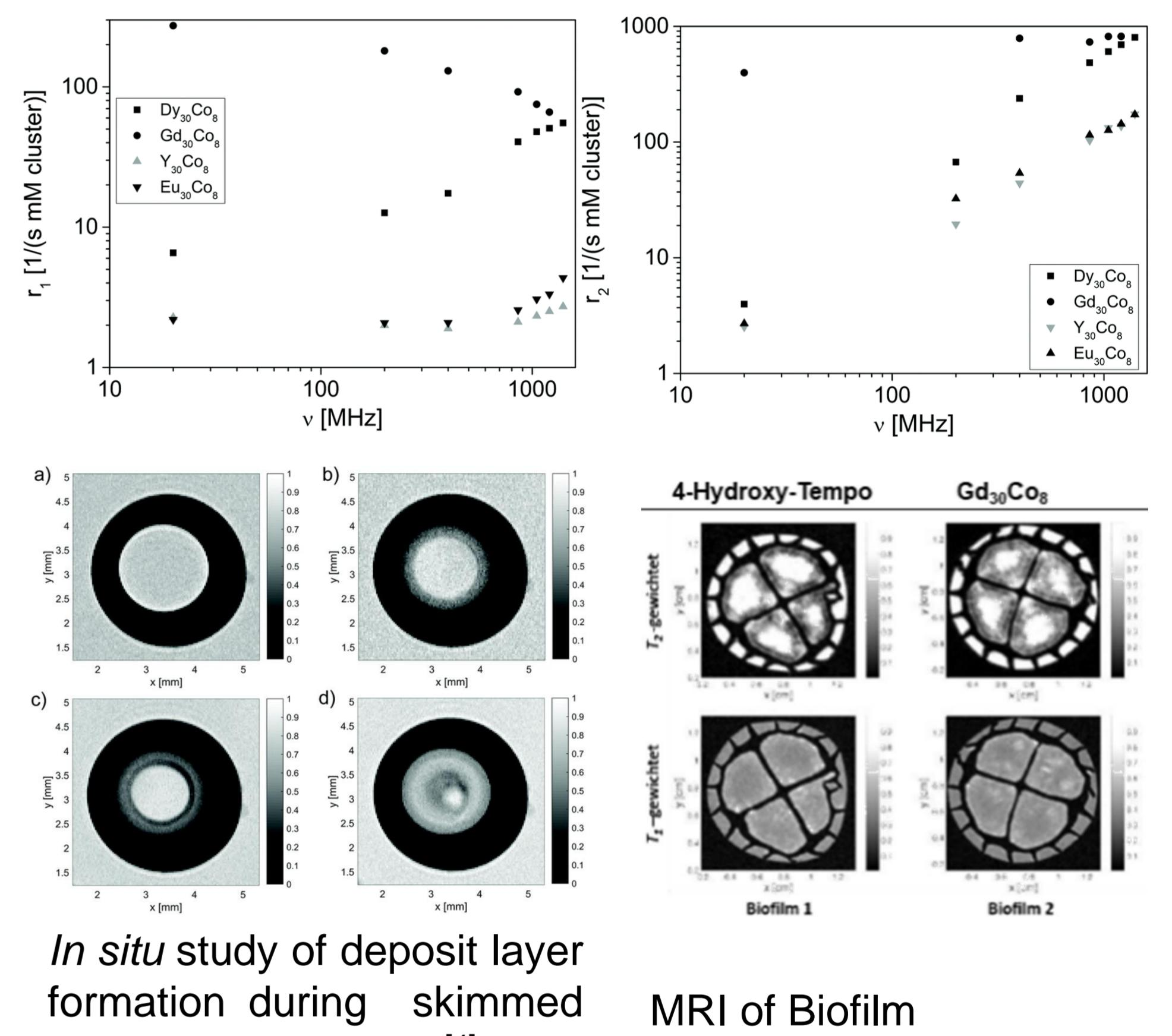
In situ study of deposit layer formation during skinned milk filtration by MRI.<sup>[4]</sup>
