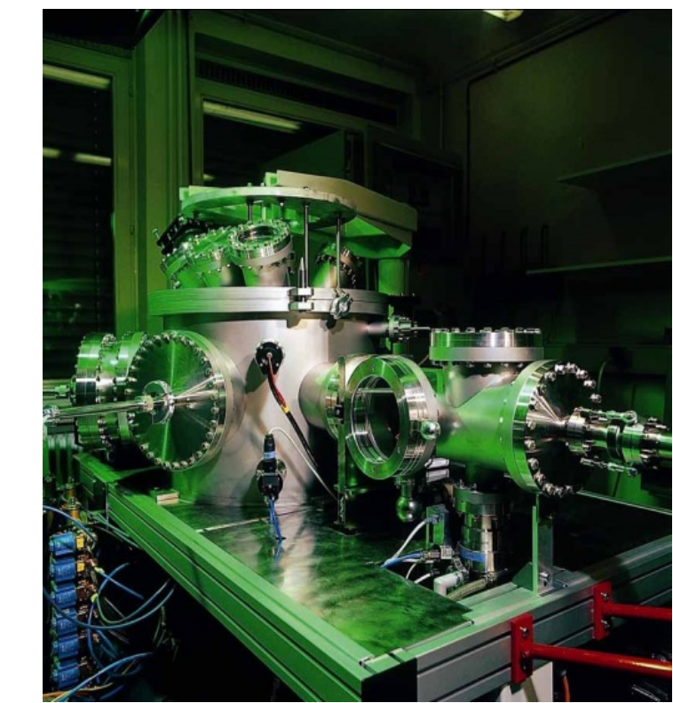
Figure 3: Sputtering facility with load lock ø 60 cm
