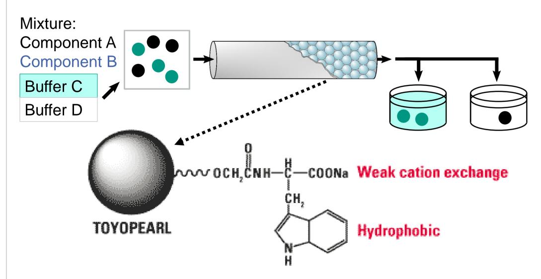
Exact chemical composition of commercial multimodal resin from TOYOPEARL is unknown, however an approximate polymer network model built from DHPMA + EGDMA + Trptophan + porogen can be established by computational molecular construction.
