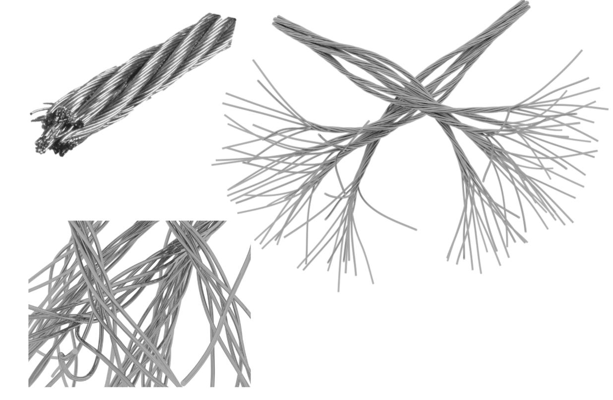
Dynamic failure of steel ropes modelled on the scale of individual wires based on Cosserat continua employing a beam element formulation. (Meier et al., 2017, Comput Methods Appl Mech Eng)
