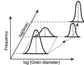
Schematic representation of the change in grain size distribution (After Detert 1978).
