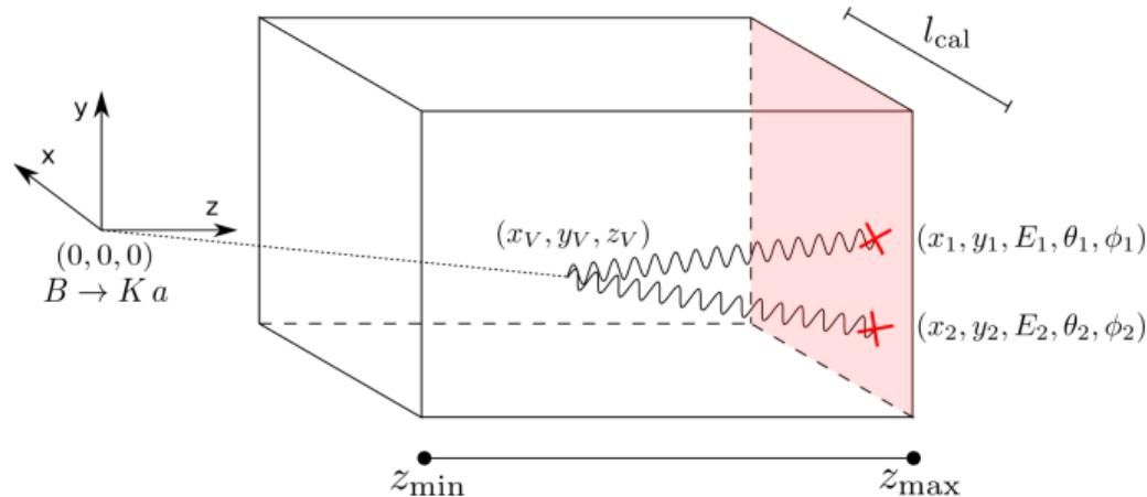
Geometry of the detector:  $z_{\min} = 10\text{m}$ ,  $z_{\max} = 35\text{m}$ ,  $l_{\text{cal}} = 2.5\text{m}$
