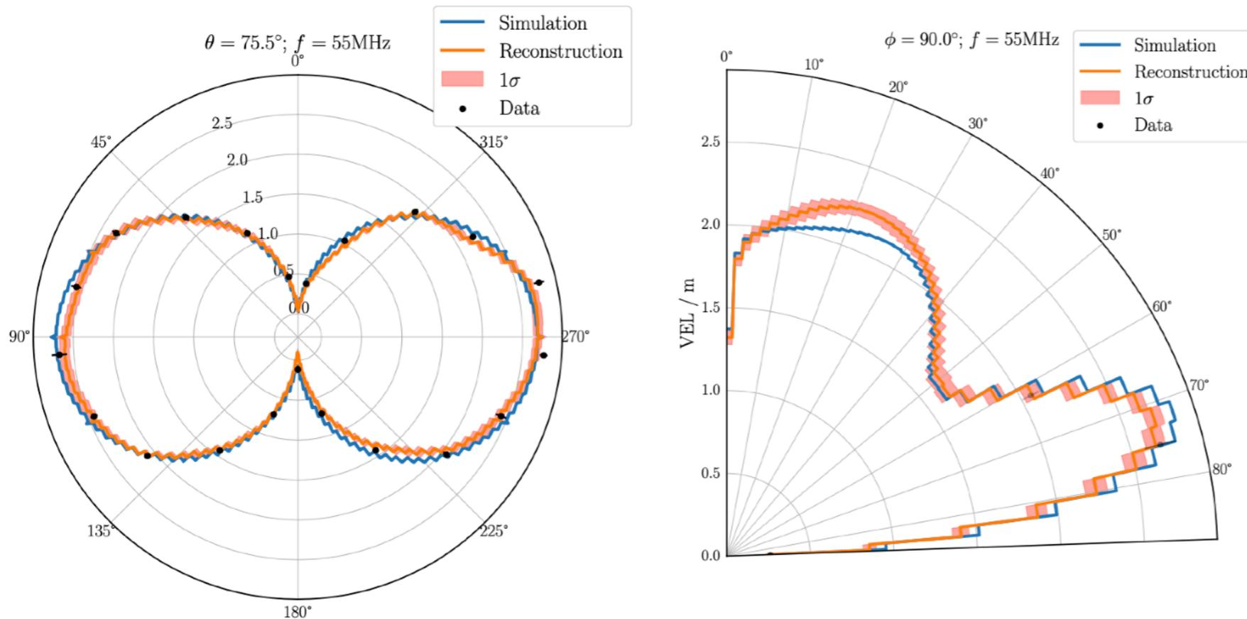
Figure 5.4: Slice for  $\theta = 75.5^\circ$  (left) and  $\phi = 90^\circ$  (right) at  $f = 55$  MHz. The black dots represent the data points, whereas their transparency represents their distance to the sliced angle. The red line with the red band shows the reconstruction and its  $1\sigma$  band. The blue line is the simulation prior.
