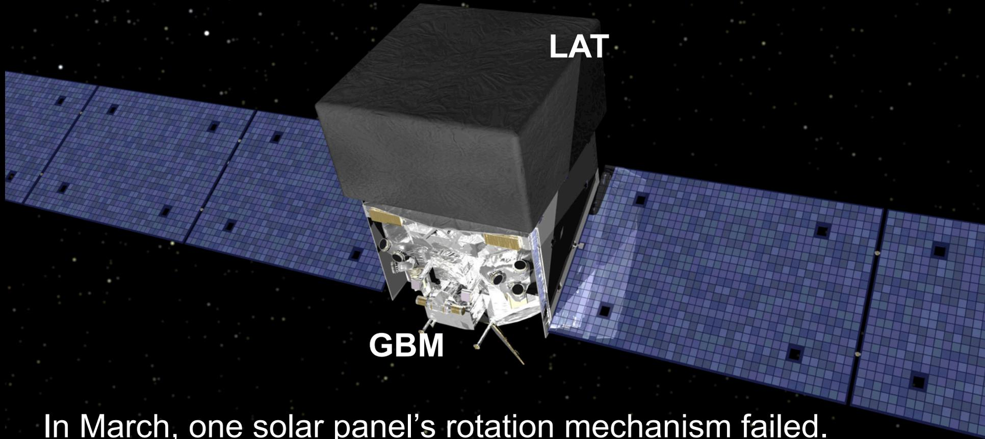
In March, one solar panel's rotation mechanism failed. The *Fermi* observing strategy for LAT changed to cover the whole sky in weeks rather than hours.
