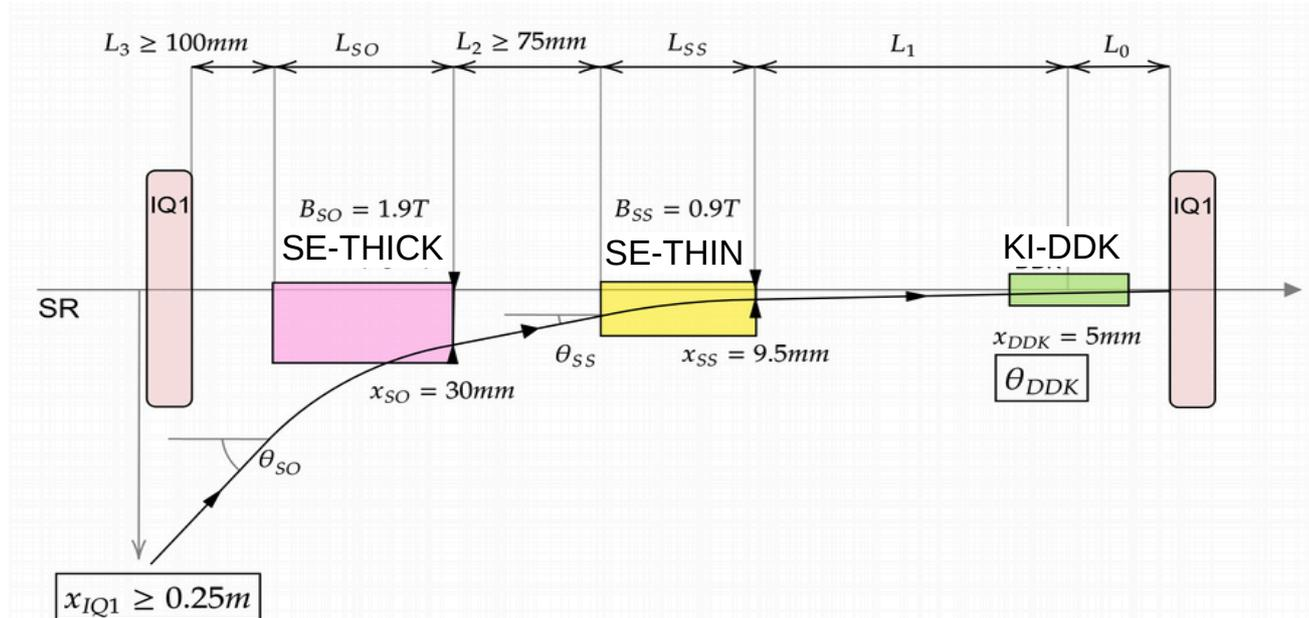
The injected beam trajectory  $x_{\text{septum}}$ ,  $x'_{\text{septum}}$ ,  $x_{\text{kicker}}$ , the kick etc. will be a trade-off among horizontal dynamic aperture, septa thickness and field, kicker apertures and pulse current/voltage...
