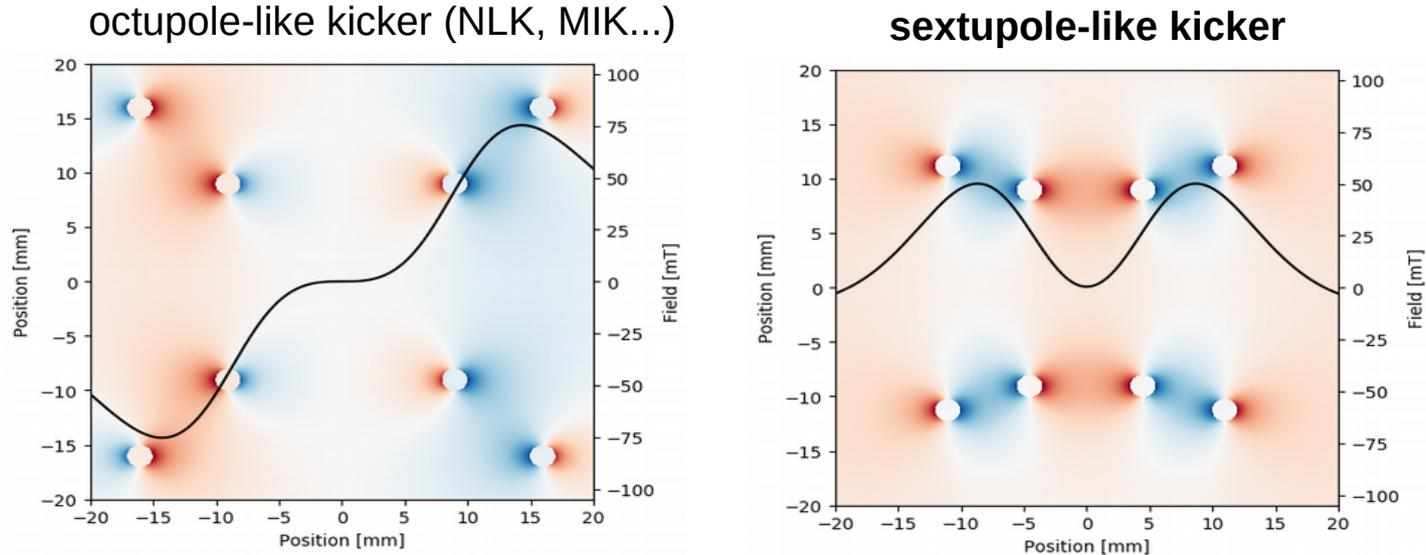
Both geometries produce a peak of the field, ideal for the injected beam position, and zero field at the centre, for stored beam transparency.
