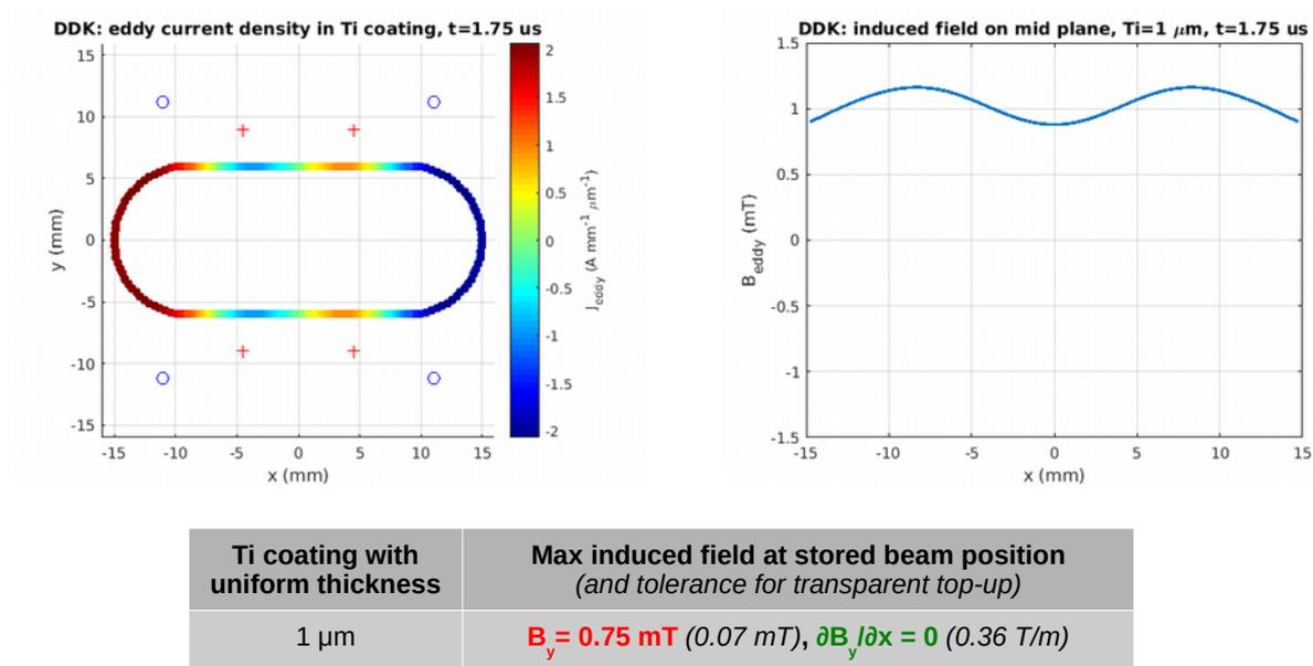
The effect of the eddy currents on the stored beam would be above the tolerances to guarantee transparent top-up.
