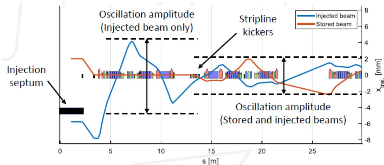
‘Trajectory of injected- and stored bunch centroids through the first achromat during single-bunch aperture sharing. Chicanes are set to a 2 mm static bump.’
