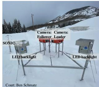
Fig. 2: VISSS at RMBL, two cameras, 90° (orange boxes), two green LED backlights (grey boxes), SONIC
