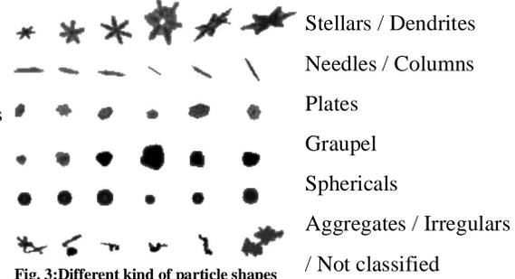
Fig. 3: Different kind of particle shapes
