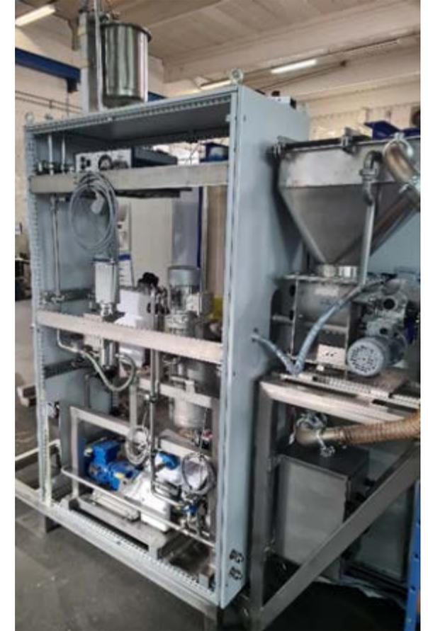
Pilot lab plant for catalyst ink mixing of IFA Technologies, Germany
