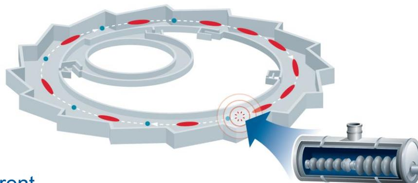
Combining two RF systems with different frequencies (1.5 GHz & 1.75 GHz) generates long and short buckets, which can be filled individually to generate optimized fill pattern.
