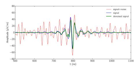
True signal and noise are identified correctly, noise is removed
