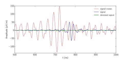
True signal is heavily distorted by noise, and removed as background
