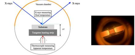
**Figure 3:** Schematic of in-situ x-ray diffraction chamber and image of a sample annealed at 1000 °C,  $2 \times 10^{-6}$  mbar
