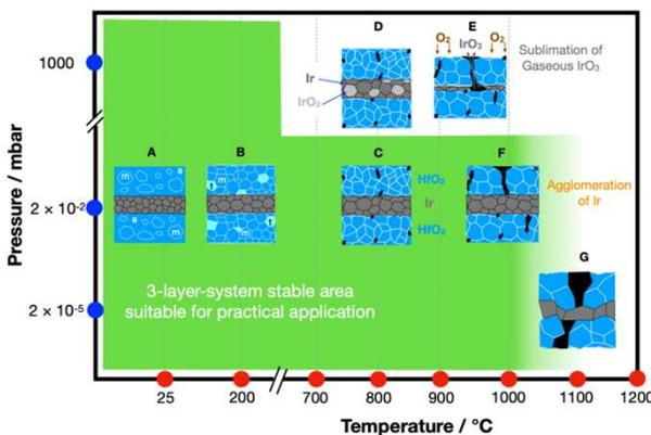
**Figure 7:** Schematic summary showing the major mechanisms and changes in an Ir 3-layer-system at different temperature and pressure ranges. The green area shows the thermally stable area of the 3-layer-system suitable for practical application.
