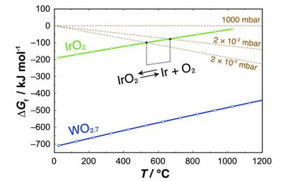
**Figure 6:** Ellingham diagrams showing Gibbs energy of oxide formation  $\Delta G$ , for IrO<sub>2</sub> and WO<sub>2.7</sub>. Equilibrium conditions of chemical reactions established at different pressures.
