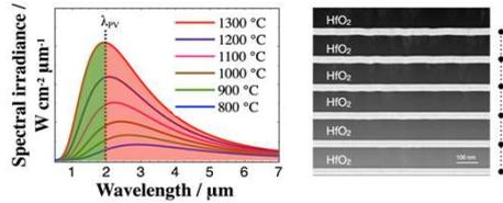
**Figure 2:** The total efficiency of the TPV system can be improved by using selective emitters which absorb long-wavelength radiation highlighted in red. On the right is the STEM cross section of an as-prepared multilayered metamaterial selective emitter
