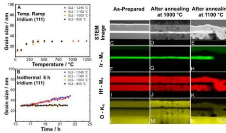
**Figure 5:** Grain size of Ir as a function of temperature and time during in-situ annealing. Cross sectional STEM-EDX images of 3-layer system before and after annealing
