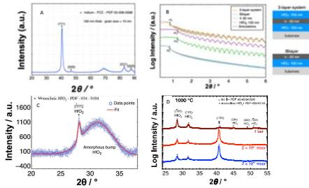
**Figure 4:** (A&C) XRD diffractograms of as-prepared Ir and HfO<sub>2</sub> layers. (B) XRR plots of various films. (D) XRD diffractograms of annealed 3-layer-systems at 1000 °C and various pressures
