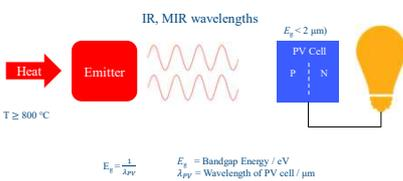
**Figure 1:** The basic working principle of a TPV system. Heat from a source is absorbed by an emitter to emit tailored radiation in the infrared regime to a photovoltaic cell that generates electricity
