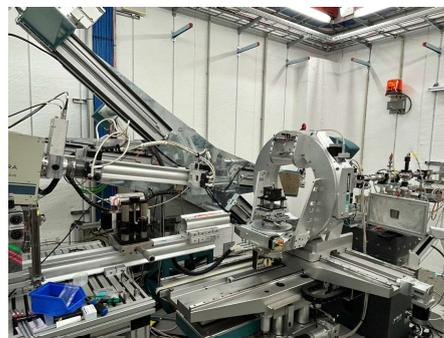
**Figure 8:** Structural and microstructural characterization of Ir-based thin films using energy-dispersive x-ray diffraction at PETRA III beamline P81A: Hereon's beamline at DESY/Hamburg
