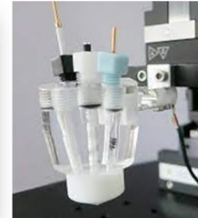
Electrochemical characterization XYZ- robot equipped with SDC
