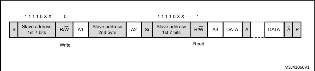
Figure 300. 10-bit address read access with HEAD10R=0
