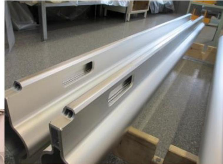
Beam pipe is made of aluminum.
