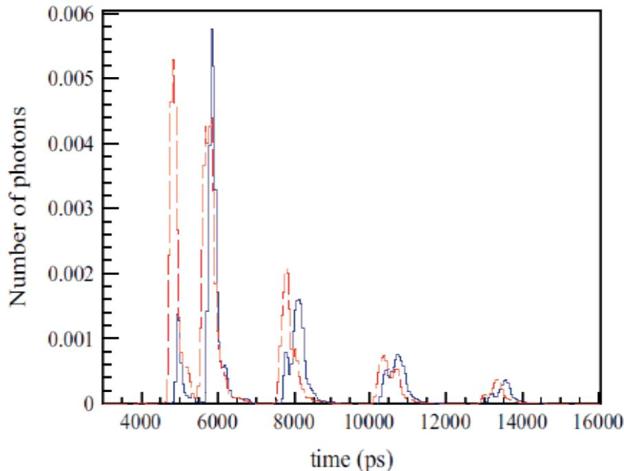
Time distribution of signals recorded by one of the PMT channels: different for  $\pi$  and K ( $\sim$ shifted in time)
