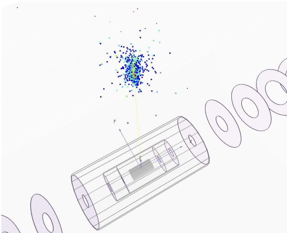
Simulated shower in the electromagnetic calorimeter of the envisioned [International Large Detector \(ILD\)](#)
