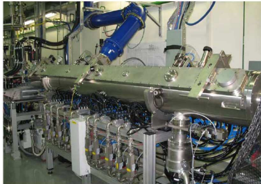
SARAF-RFQ: 3 MeV D + , res. frequency: 175 MHz, 250 kW CW
