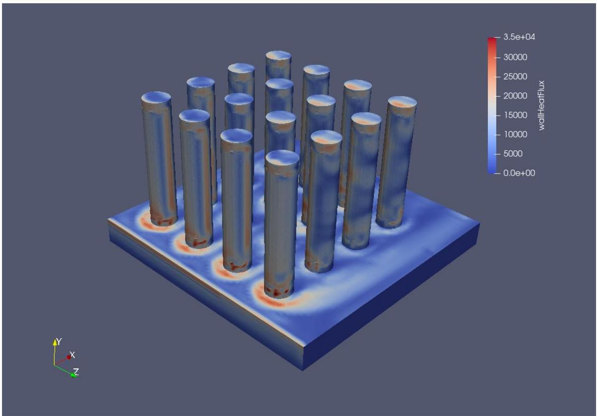
*Fig.8 Wall heat flux at surface of pins and plate (in W/m<sup>2</sup>)*
