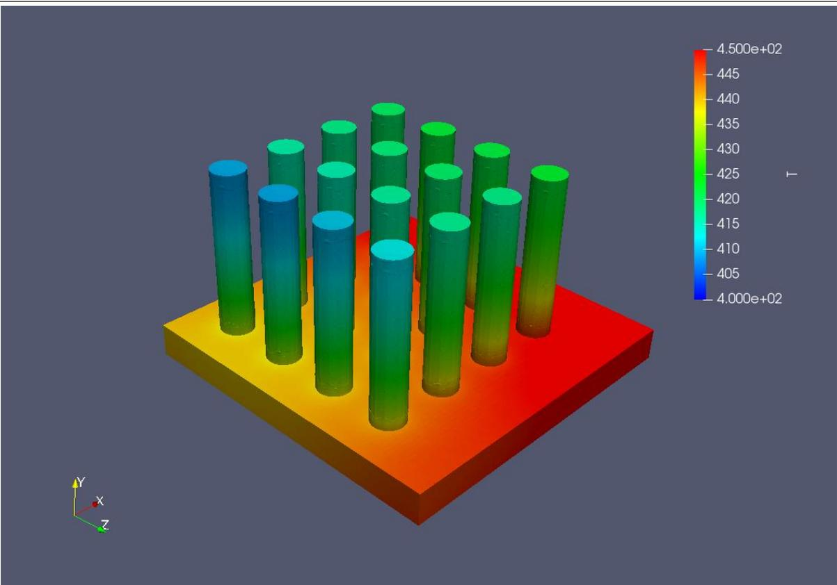
*Fig.9 Temperature distribution at surface of pins and plate (in K)*
