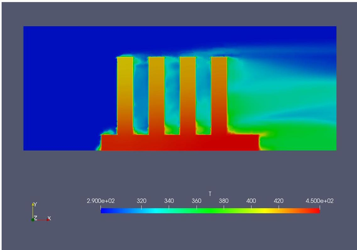
Fig.10 Temperature distribution of passing air flow (in K)
