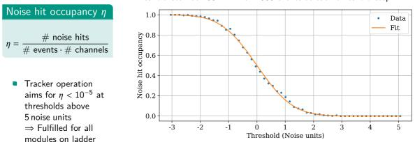
Threshold scan at 100 kHz with 1000 events at each threshold step
