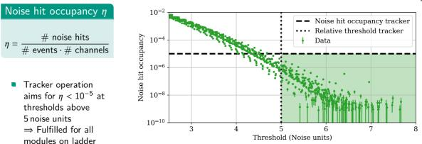
Threshold scan at 597 kHz with about 100 000 events at each threshold step
