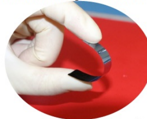
Thin Si with integrated heaters
