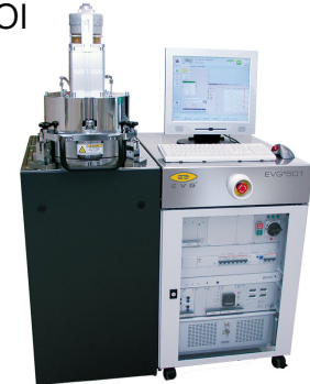
Direct and adhesive (temporary) bonding: EVG501
