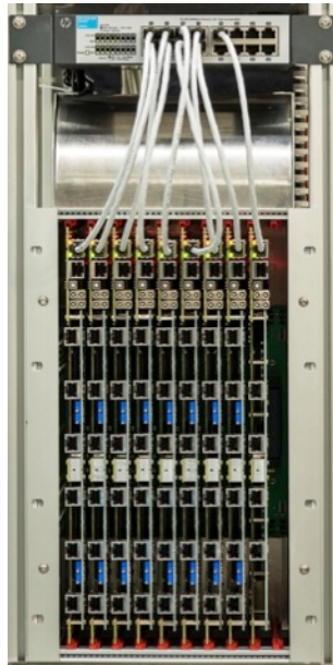
Electronics crate serving up to 192 pixel
