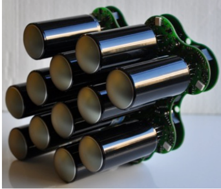
144 pixel PDP test setup
