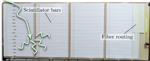
Inlay: Scintillators with wavelength shifting optical fibres
