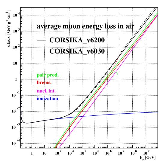
Average Muon Energy Loss in Air at Sea Level.
