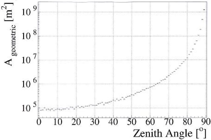
Geometric collection area vs. zenith angle for HEGRA CT1 (Schröder). (HEGRA CT1 was precursor of MAGIC Cherenkov telescope).
