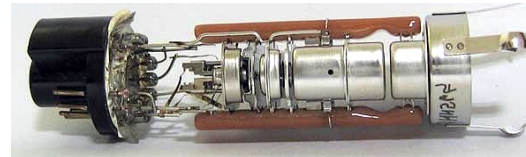
Cathode ray tube of an electron gun
