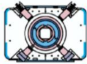
TEVATRON B = 4 \text{ T} Bore : 76 mm
